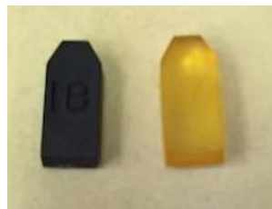
Figure 3.16: Cured resin in trapezium shape for TEM analysis
