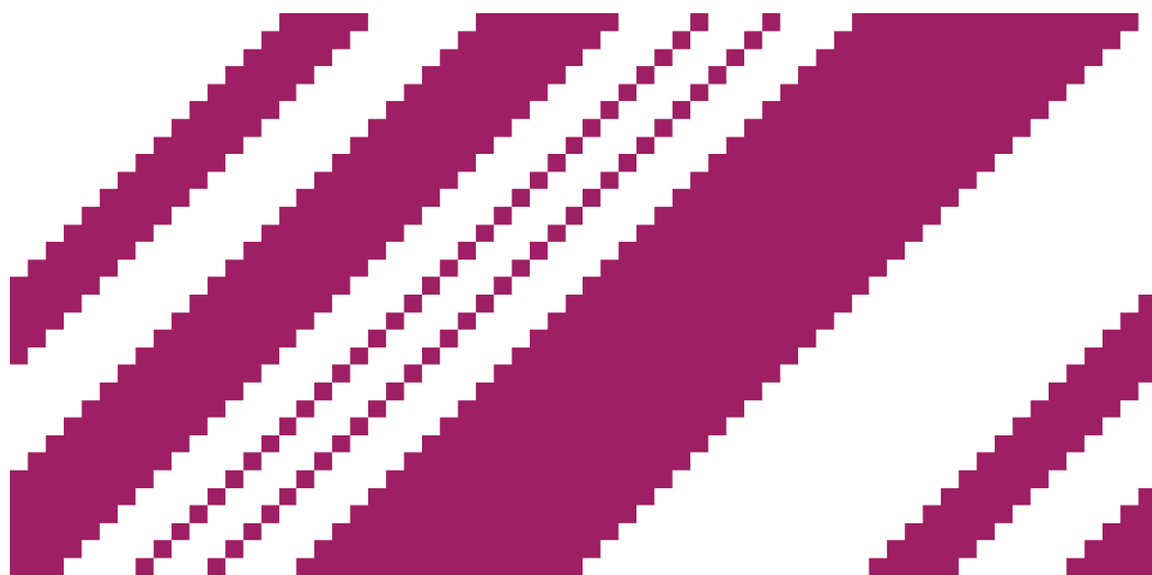
Figure 2.8 A run of rule 138. The cell space wraps round horizontally, so the diagonal lines on the right side of the run continue on the left.
