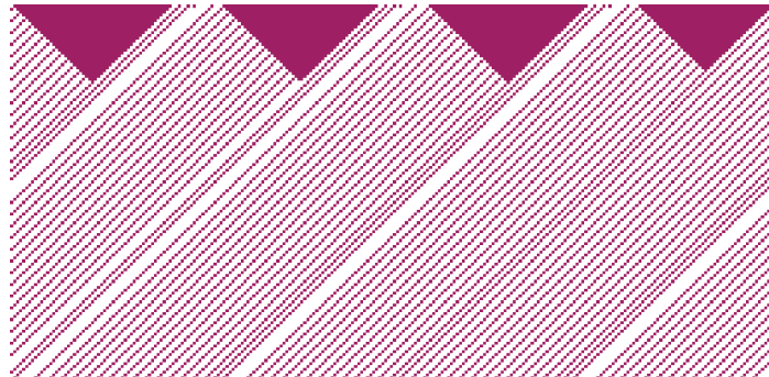
Figure D.1 Rule 130 showing a segment of the initial condition described in this section. The phase transition takes place at step 26, the time at which the triangles disappear.
