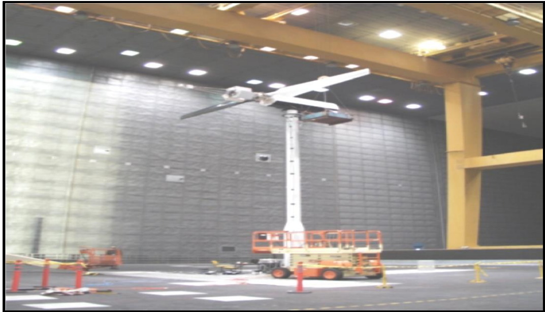
Figure 4-1 The NREL phase VI rotor in the NASA – Ames wind tunnel (Hand et al. , 2001).
