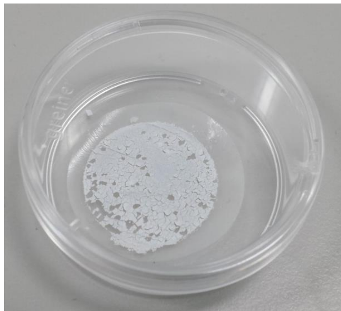
Figure 3.15. Filter membrane with isolated silicon nitride particles deposited on the surface, which have formed a cracked layer. The initial doping volume was high ( 1 \text{ mm}^3 ).
