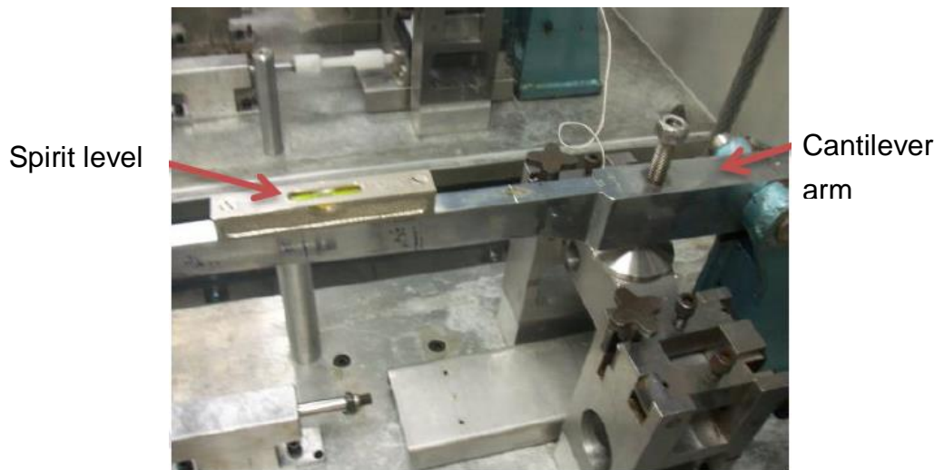
Figure 2.3. Load calibration of the pin-on-plate machine. A. Setting up the load cell and flat ended load screw. B. Use of a spirit level to ensure horizontal positioning of the cantilever arm.
