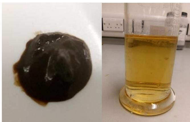
**Figure 50:** (left) TEPR residue obtained after filtration; (b)  $H_2O$  diluted  $bmim[HSO_4]$  after filtration.
