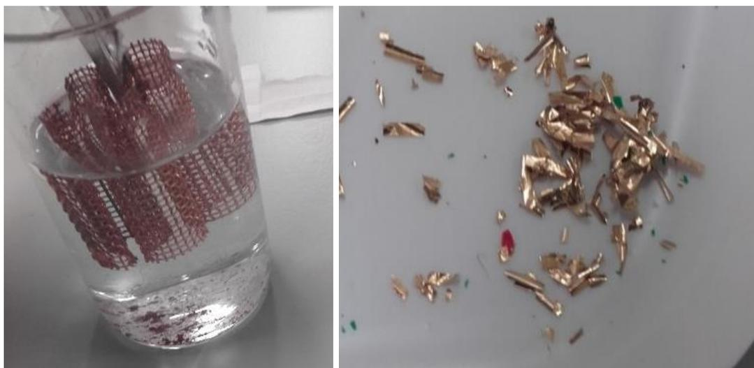
*Figure 74: (a) The copper mesh used as cathode, copper-nickel alloy powder dropping off copper mesh into distilled water; (b) some gold flakes collected after Cu-Ni leaching process.*
