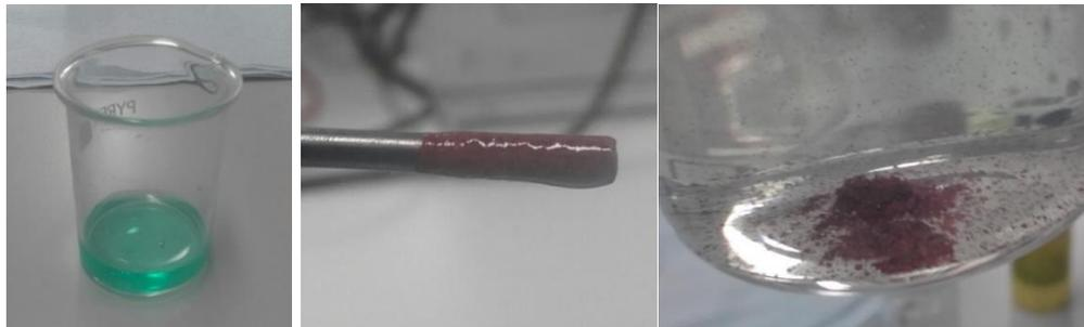
*Figure 68: (a) Leachate from Cu-Ni leaching used as electrolyte; (b) Cu-Ni alloy deposited on a graphite electrode after electrodeposition step at 3V for 3mins; (c) Cu-Ni alloy deposits being washed in distilled water.*
