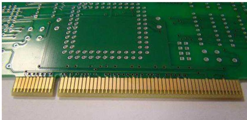
**Figure 4:** *Gold plated edge connector (PCB finger) [57].*
