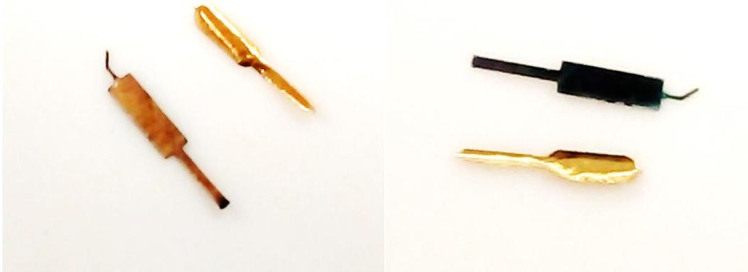
*Figure 58: A comparison between a rigid multi-layered surface plate before leaching and a gold flake after leaching reaction: (a) a top view of the surface plate compared to a gold flake; (b) a bottom view of the surface plate compared to a gold flake after leaching away copper and nickel layers.*
