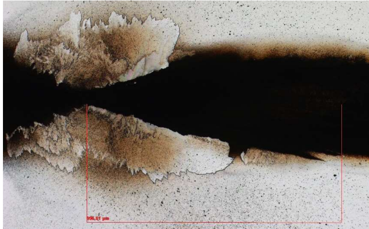
Figure 4.1: Ablation crater generated by rastering the material surface in the beam path with changing z-axis.
