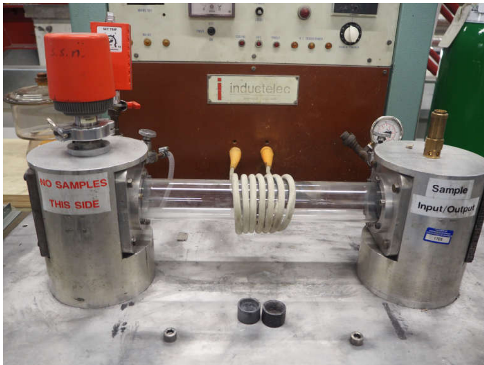
Figure 2.3 small scale melter used to prepare alloys with volatile or low melting point components
