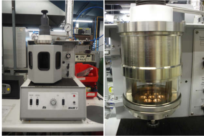
Figure 2.2 Buhler Mini Arc Melter the hearth on this model is suitable for melting up to 6 alloy ingots at one time, the pumping system consists of an oil free scroll pump and high vacuum turbo molecular pump
