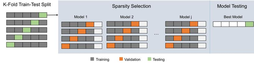
**Figure 4.1.** A diagram of the nested k-fold cross-validation with model selection.
