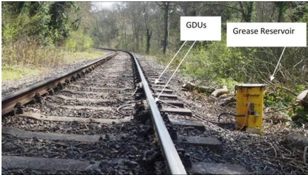
Figure 22- a typical wayside GDU [68]
