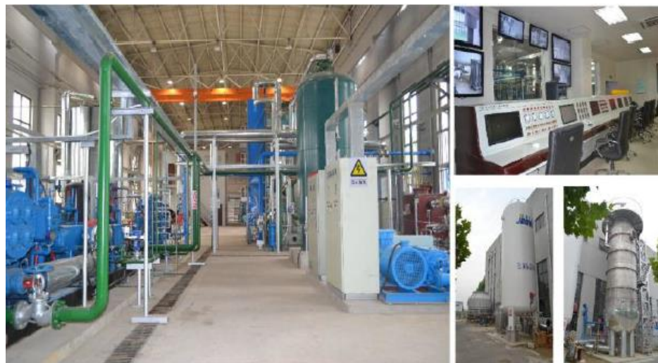
Figure 2-6. A 1.5MWe SC-CAES pilot plant (Wang, 2017).
