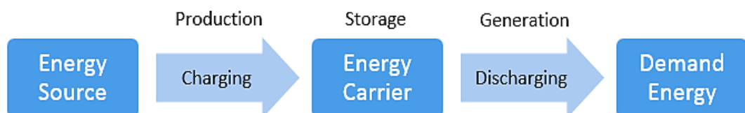
Figure 1-3. The schematic concept of energy storage (Aneke and Wang, 2016).
