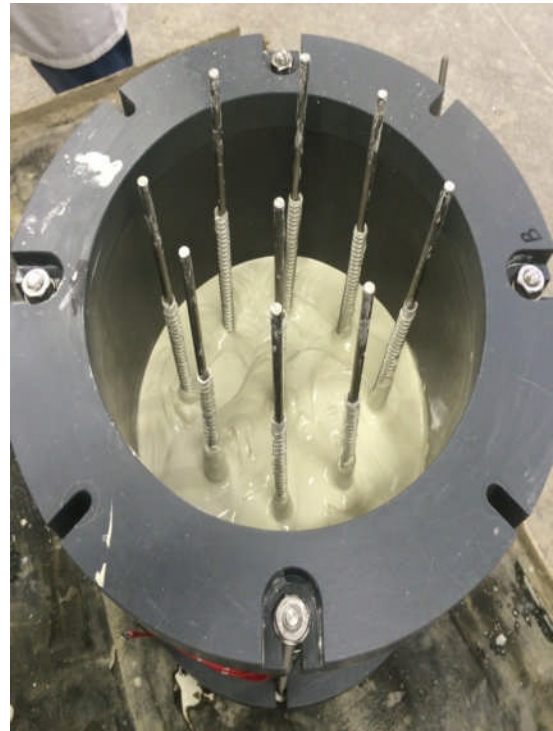
(b) The first prior to vibration with the steel rods inside supporting the electrodes
