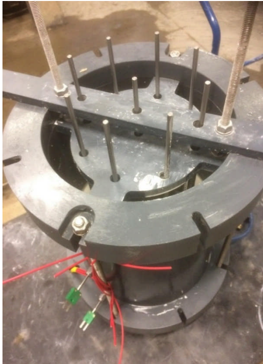
(a) Holding the springs in place while the first layer was placed
