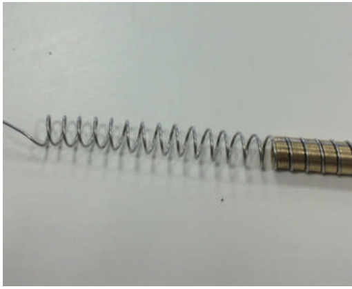
(a) coiled spring electrode
