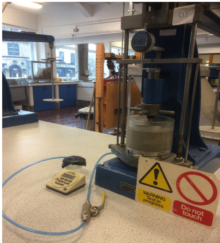
Figure 4.3 (b) General arrangement of the consolidation cell used in control tests
