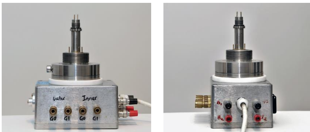
Figure 4-5. A side view of the reactor showing gas (left) and electrical (right) connections (GI – gas in, GO – gas out, B1 & B2 – bottom pins, and T1 & T2 – top pins).
