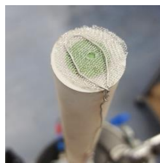
Step 4 – Place a current collector with a mesh on top of the cell.
