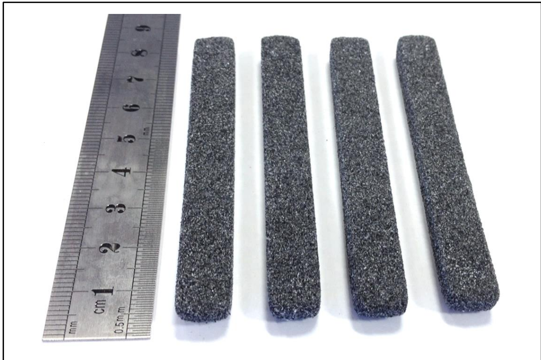
Figure 7.17 : Laser sintered flexural test samples produced at laser power of 12 watts
