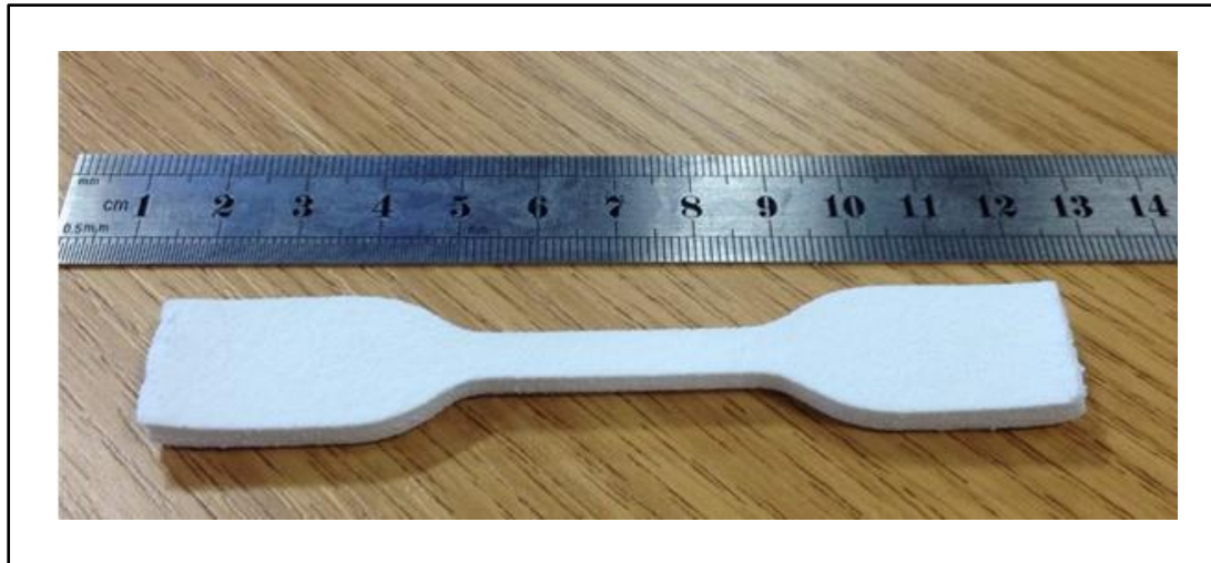
Figure 5.16: Sintered UHMWPE part fabricated using 10 watts laser power
