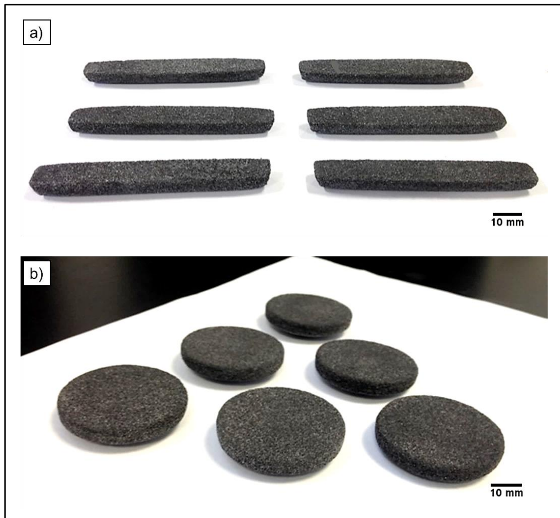
Figure 7.16 : AC-UHMWPE test samples produced at laser power of 8 watts a) Three point bend samples, b) Water flow rate test samples
