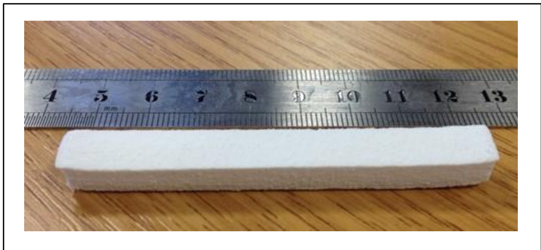
Figure 5.2: Sintered part of UHMWPE fabricated using 10 watts laser power
