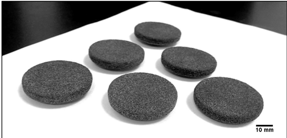
Figure 9.14 : 3D printed disc-shaped filters using laser sintering
