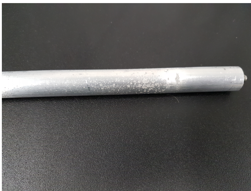
Figure 6.18: Arc points on inner rod of final transmission line in the Blumlein transmission line, caused by arcs through air bubbles trapped in the laser tank.
