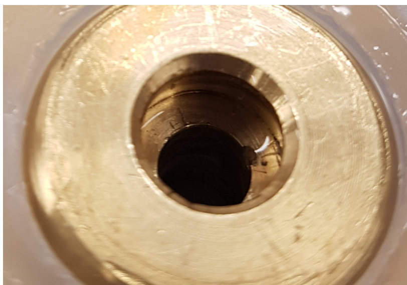
Figure 6.21: Photo of the scratches on the brass electrode which allowed for an arc point to form.
