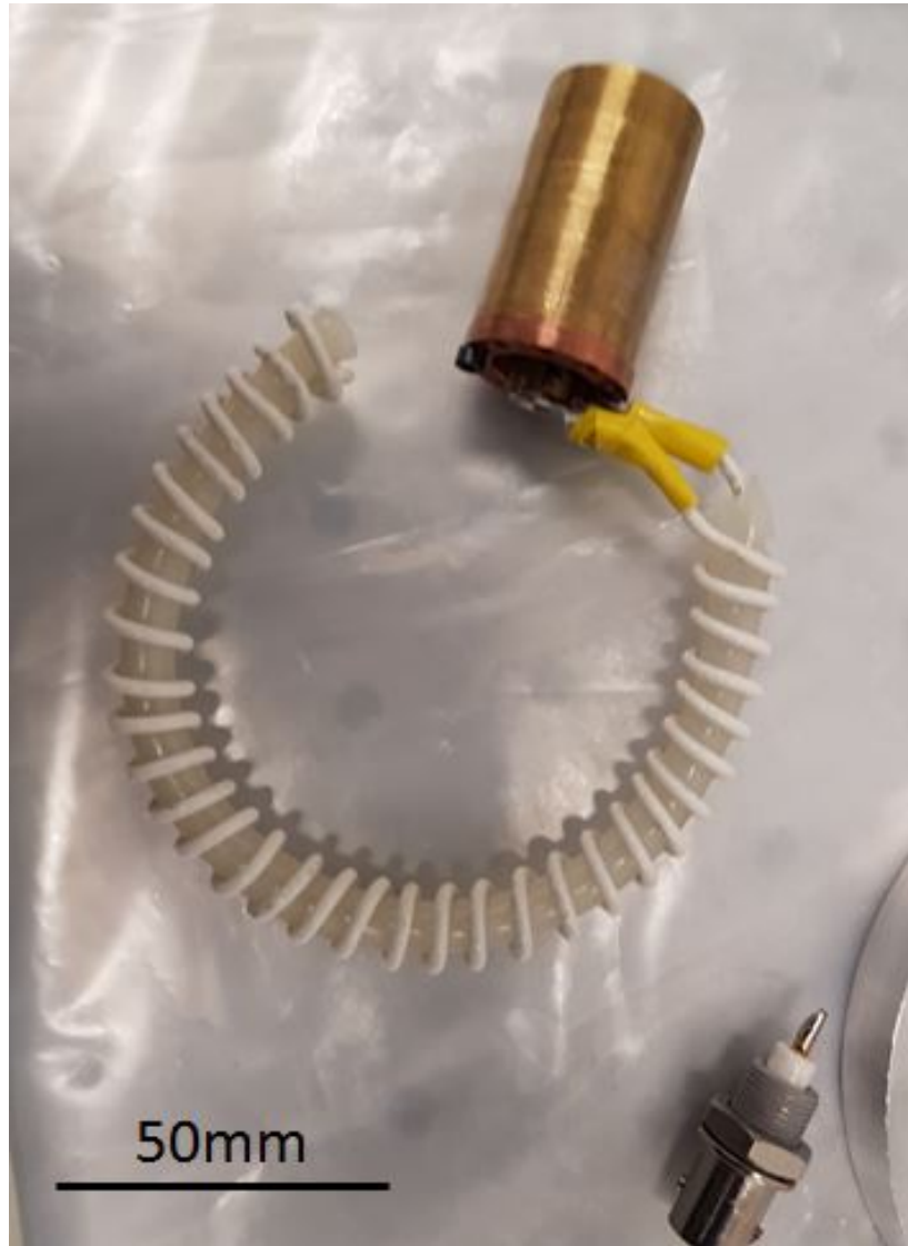
Figure 5.7: Photo of the Rogowski coil installed in the capillary discharge laser, which consists of a helical coil of wire with one end returning through the centre of the coil to the other end, so that both terminals are at the same end of the coil.
