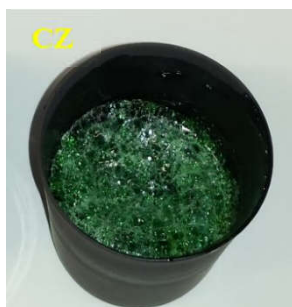
Figure 7.2a CZ glass after corrosion test in Inconel 601 crucible
