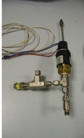
Figure 4-11 The pressure relief valve.
