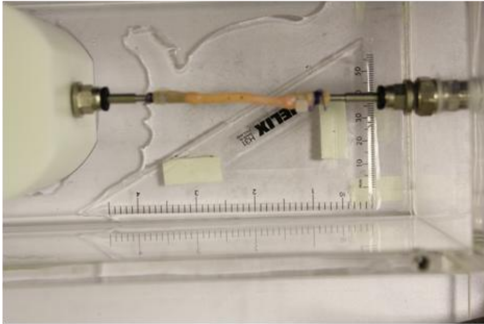
Figure 3.3: Illustration of the artery mounting on the pressure rig. The artery was fixed on both ends, using sutures and cable ties on specially designed stainless-steel bars with a bore of 2mm to allow water to pass through. The white block at the left of this image is solid, and since fluid cannot go through, it allows the dilation of the artery.
