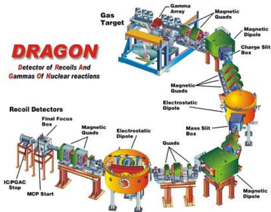
FIGURE 3.8: Diagram of the DRAGON facility at TRIUMF. Image taken from http://dragon.triumf.ca/system.html
