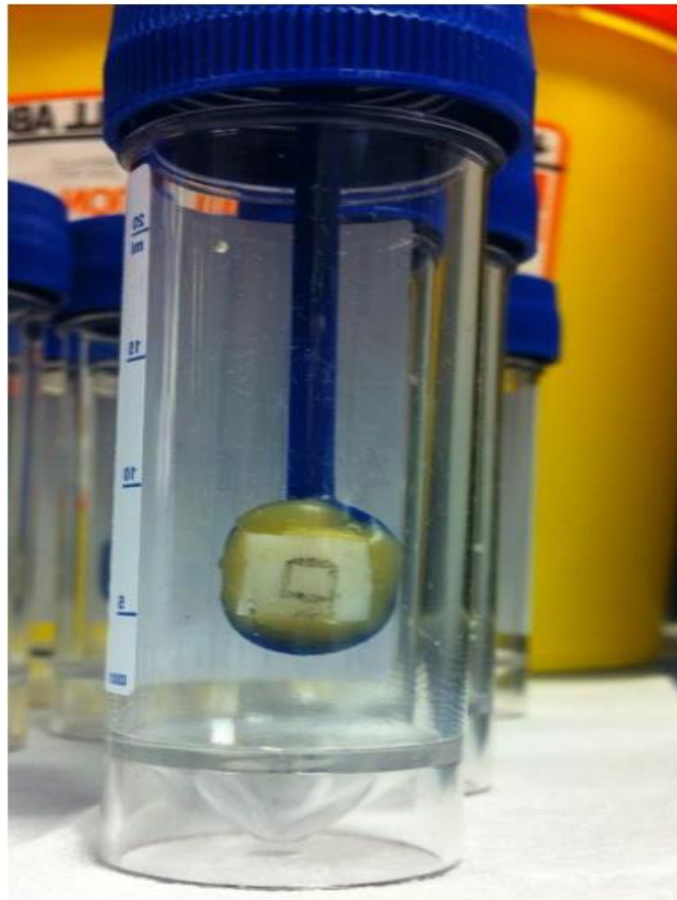
Figure 2: Enamel slab attached to the plastic spoon with sticky wax and suspended in the plastic universal tube
