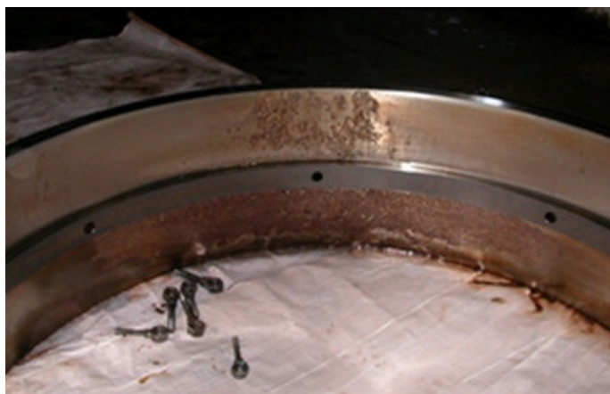
Figure 2-3 Fatigue wear in a roller bearing [26]
