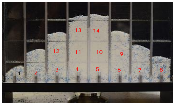
Figure 3.25: (A) Different stages of sample extraction in ternary heap (B) grid marked heap.
