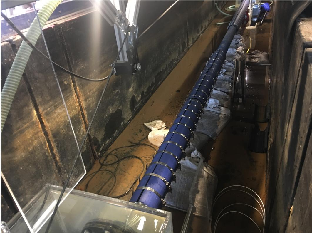
**Figure 3.6:** Experimental setup for 5m metal pipe: The hydrophone pulser and receiver unit, H8103, travels up and down a one metre steel pipe that is immersed in water. Experimental recording was conducted on a 40 cm mid-section of pipe.
