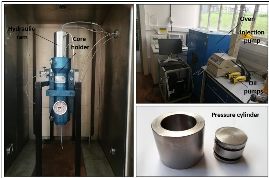
Figure 4-8: Photograph of Field's metal injection experiment setup.
