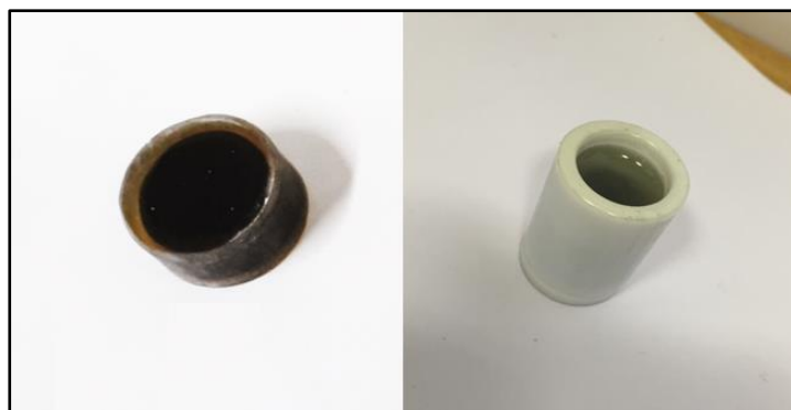
Figure 5-7: Teflon mould and sample after sealing placement
