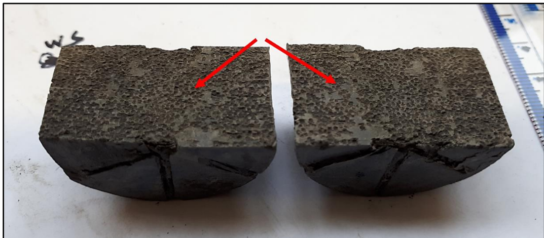
Figure 6-13: WS sample fracture walls after performing the experiment showing impressions of the proppant embedment into fracture wall.
