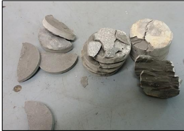
Figure 1-2: Picture showing clearly the delamination problem.
