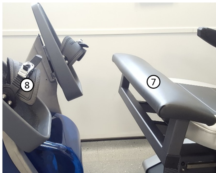
Figure 2.1: Eccentric recumbent stepping ergometer (BTE, Hanover, MD, USA; http://www.btetech.com/product/eccentron/ ). A reclined seat (1) can be moved forwards and backwards along rollers (2). The foot plates (3) are driven backwards and forwards by a motor housed within the main casing (5), and the load cells (4) are positioned behind each foot plate. A touch screen (6) is visible to the participant and can be connected to external computers to customise the display. Additionally, an adjustable under knee support (7) helps to further prevent knee hyperextension and foot straps were added (8) for additional participant comfort and stability. To produce concentric contractions, the participant was instructed to push the foot plates as they move away from them (black and blue arrows). To produce eccentric contractions, the participant was instructed to resist the foot plates as they moved towards them (black and red arrows).
