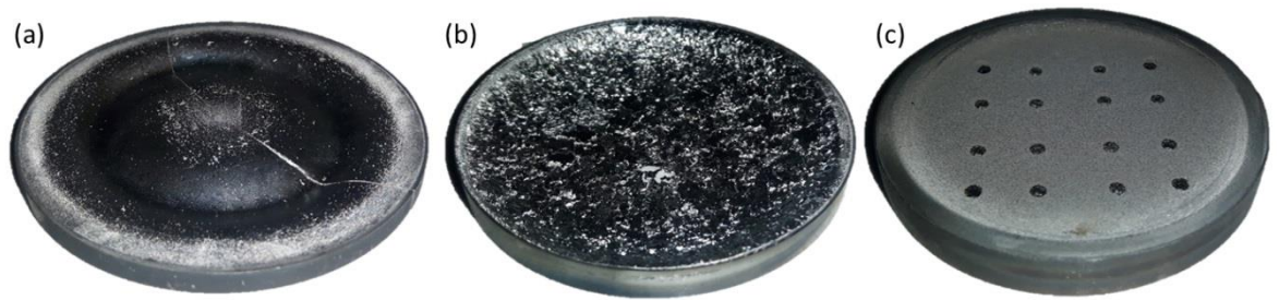
Figure 6.4 - (a) Used magnetron target with erosion 'racetrack'. (b) Alloy HiTUS target with high utilisation (0 mm thickness at centre 6 mm at edges) (c) Powder pressed HiTUS target with holes to allow doping pegs to be inserted.
