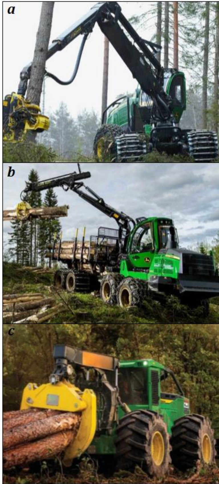
Figure 3.11 – Examples of forest machines, utilised in the felling and extraction processes; a) John Deere 1470G wheeled harvester, b) John Deere 1510G forwarder, and c) John Deere 948L grapple skidder [105]
