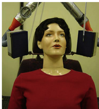
FIGURE 2.13: Image from Melikov et al. [2012] showing the breathing thermal manikin and the placement of air terminal devices.
