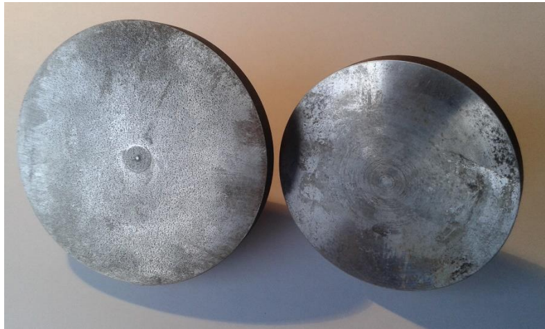
Fig: 3-1: The image shows the concentric ring pattern on the mounting plates produced during the manufacturing process. Marks and patina can be seen from the corrosion of the plate material due to the interaction with the water content of the gelatine, emphasising the need for regular cleaning.
