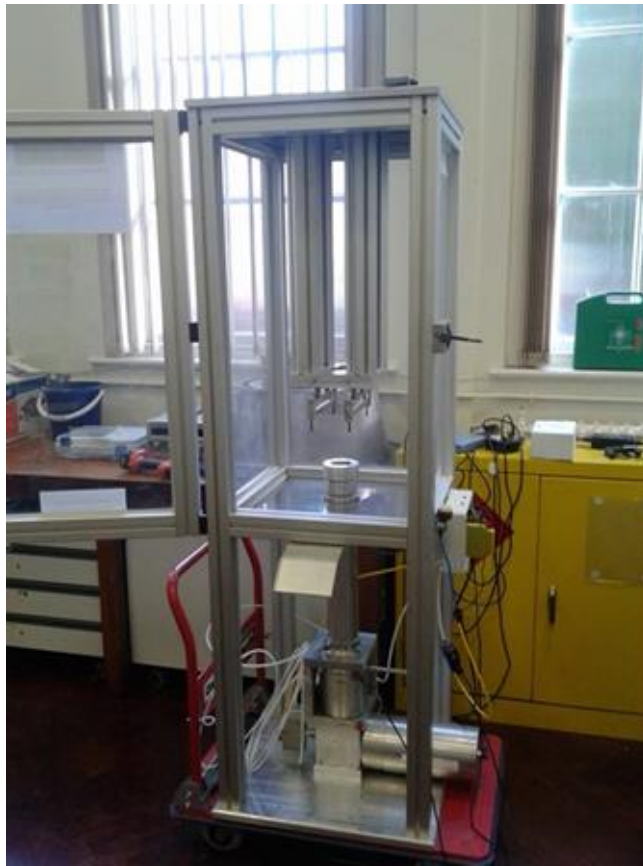
Fig: 6-2: The cannon in the lab the mounting plate can be seed suspended from the frame and the ballistic shield can be seen surrounding the barrel aperture, with the compressor tank seen below the cannon body.
