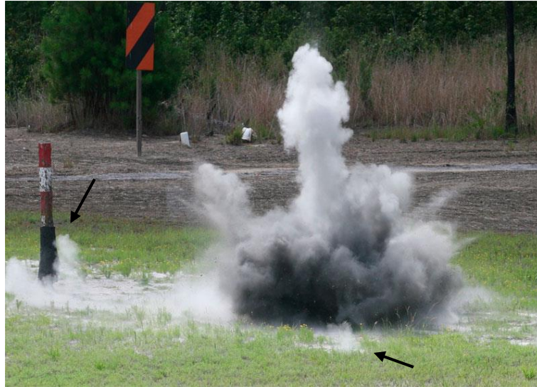
Fig: 2-2: Detonation of a hand grenade. The dust and gases can clearly be seen expanding from the point of detonation. The black arrows indicate where the initial shock wave that generates the rapid change in pressure has interacted and kicked up dust ahead of the main dust and smoke cloud from the explosion [94].
