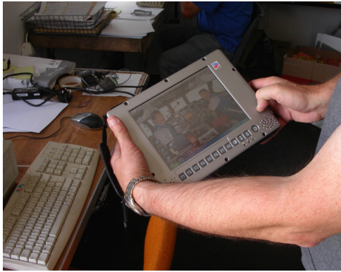
Figure 27: Left: Mike Rains holding the ruggedised tablet PC tested in the field at Silchester. Though designed for outdoor military use and by far the most expensive of the models tested, the screen was so dim it was virtually useless (Rains pers. comm. July 2006). Right: Working in the Silchester field office with data drawn on a far less expensive, but better performing tablet PC. Photos by the author.
