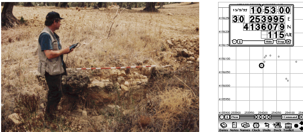
Figure 23: Left: Screenshot of the capture of vector-based spatial data within FieldNote on the Apple Newton. Right: Nick Ryan testing the MCFE system in the field, wearing a GPS device with a hat antenna, attached to an Apple Newton handheld computer. Reproduced from FieldNote: extending a GIS into the field (Ryan et al. 1999).
