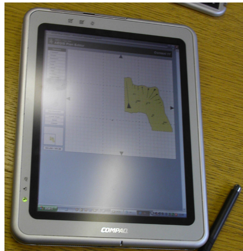
Figure 28: Left: The IADB on a handheld PC, which also has vector drawing capabilities. Right: A tablet PC showing the SVG-based vector drawing program which mimics the grid of a planning frame, and allows for drawings made in plan view to be instantly available within the database as soon as they are saved. Photos by the author.
