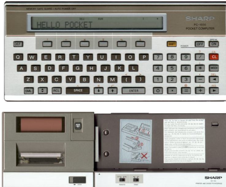
Figure 22: First manufactured in 1982, the Sharp PC-1500 Pocket Computer, and its four-colour printer dock, was likely the first handheld computer used for digital field for recording in archaeology. Photos from the Pocket Computer Museum (Laroche 2010). Reproduced with permission.
