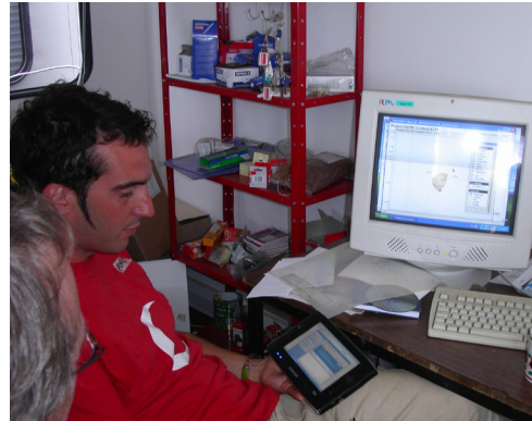
Figure 27: Left: Mike Rains holding the ruggedised tablet PC tested in the field at Silchester. Though designed for outdoor military use and by far the most expensive of the models tested, the screen was so dim it was virtually useless (Rains pers. comm. July 2006). Right: Working in the Silchester field office with data drawn on a far less expensive, but better performing tablet PC. Photos by the author.
