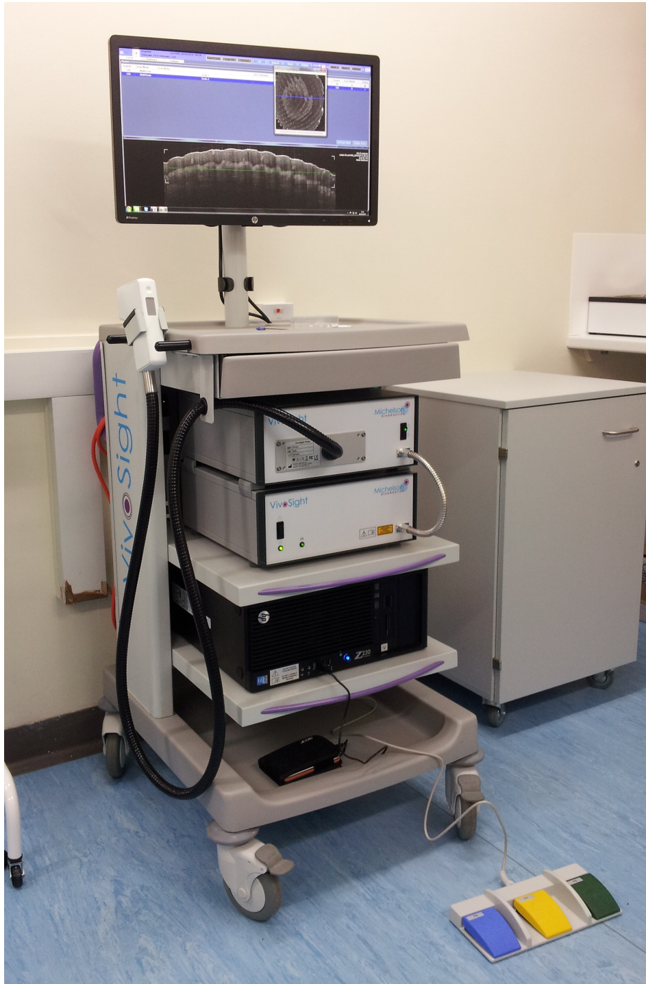
FIGURE 2.1: Vivosight OCT system with handheld optical probe
