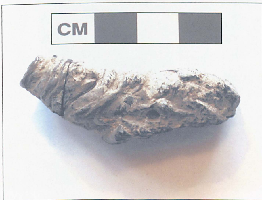
Plate 4.8 Fragment of tap slag from Chrysokamino probably corresponding to a "runner".
