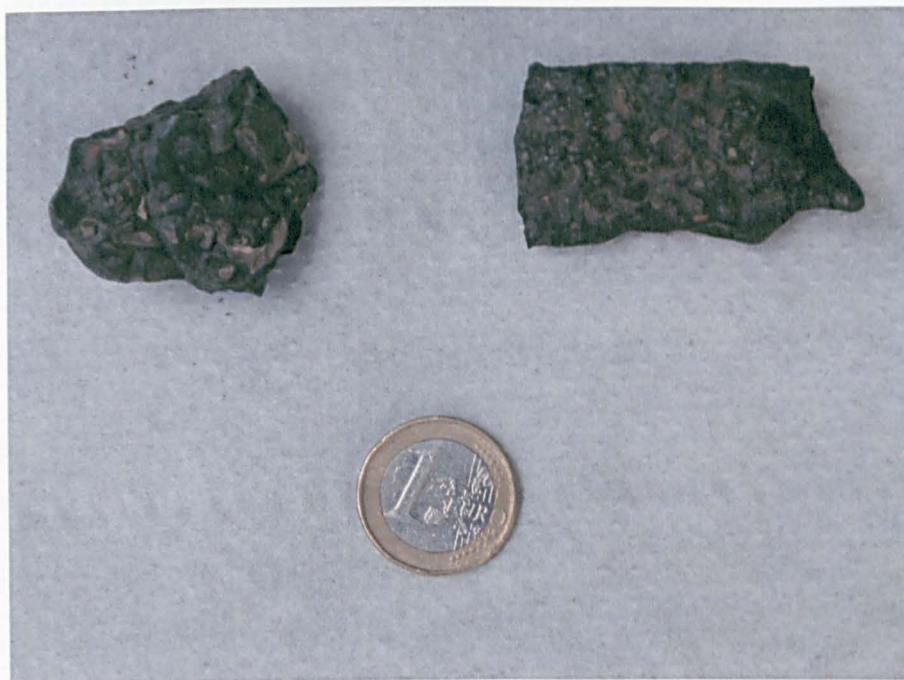
Plate 4.7 Fragments of tap slag from Chrysokamino with pieces of rock adhering on their lower surface.
