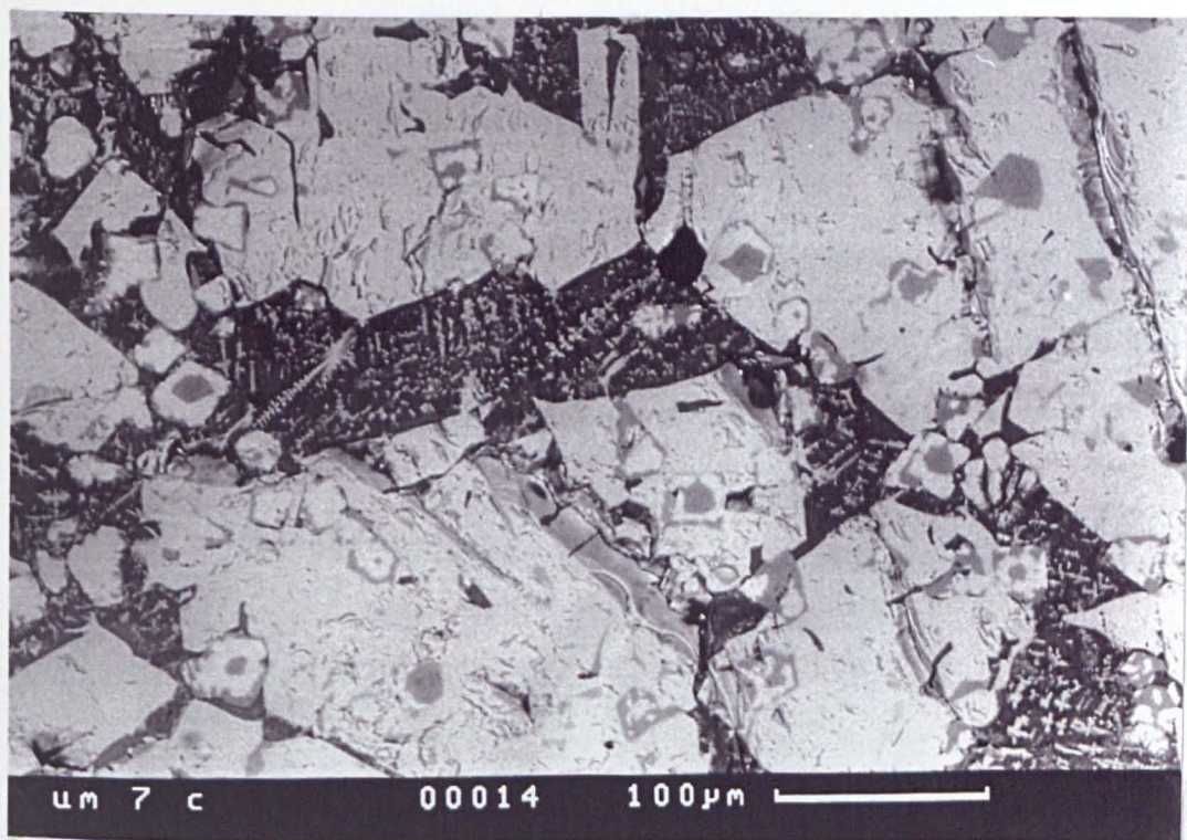
Plate 5:4 Fine rods of light grey fayalite in glass matrix containing light grey broken fayalite and dark grey euhedral crystals of hercynite.
