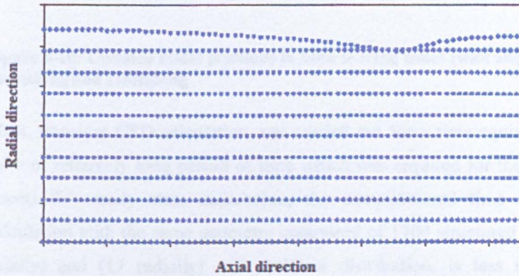
Figure 5-9: The occurrence of negative volume due to the intersection of moving wall and the first grid line of bulk fuel
