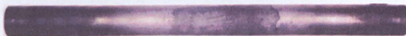
Figure 4-7: Typical Jet Fuel Feed Arm Injector Used for Heated Nozzle Module in AFTSTU
