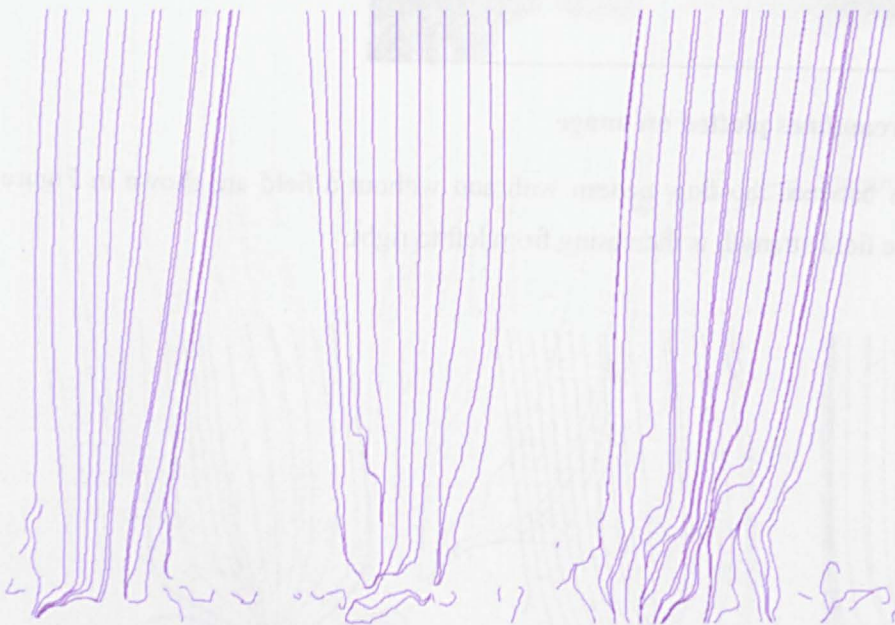
Figure 6.38 Comparison of rich flame no field, 5kV and 10kV (left to right)
