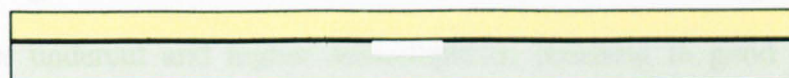
Step 8: Bonding with a piece of glass at the top of the channel
