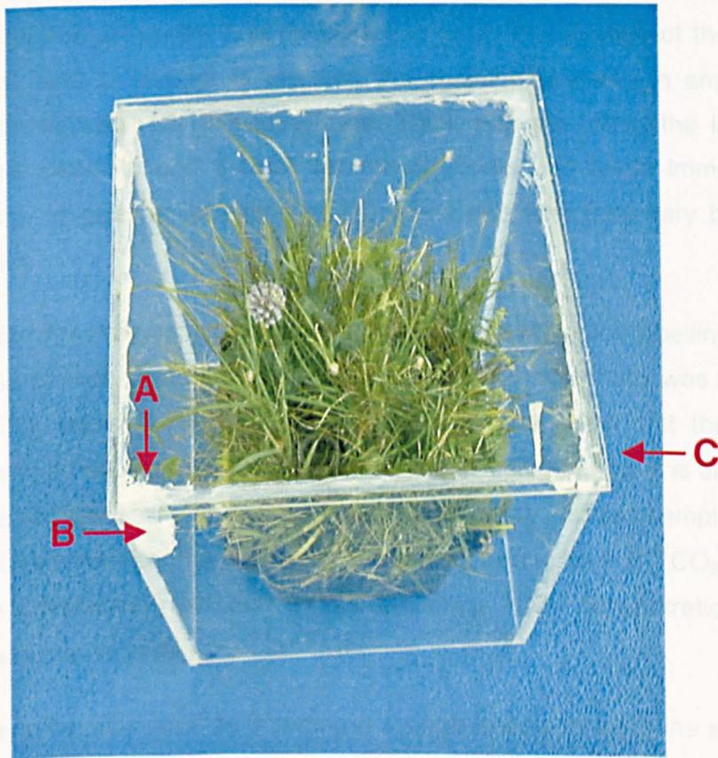
**Fig. 5.3** Micro-turf shown inside labelling chamber. Arrow A shows labelling hole, arrow B shows cuvette inside chamber, arrow C shows gas sampling hole.
