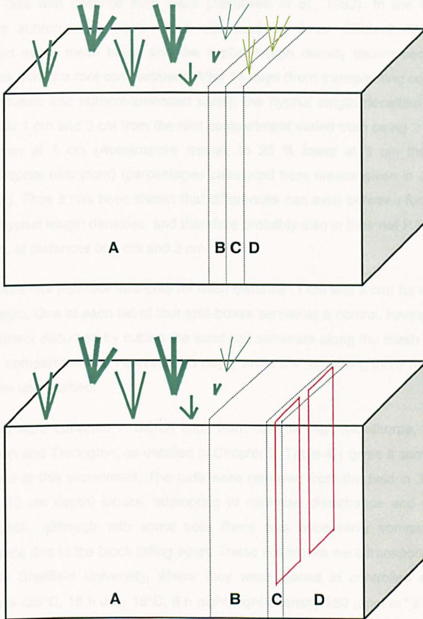
**Figure 4.1** Diagrams of split-pots. The box dimensions were 12 x 21 x 15cm (width, length, depth); the turf compartment **A** measured 12 x 12 x 15cm (width, length, depth). Compartment **B** was either 1 cm or 3 cm long; compartment **C** contained either bioassay seedlings or membranes. These split-pots were specially constructed using PVC plastic and Tangit™ All Pressure glue (ASTM D-2564 from Henkel KGaA, Germany).
