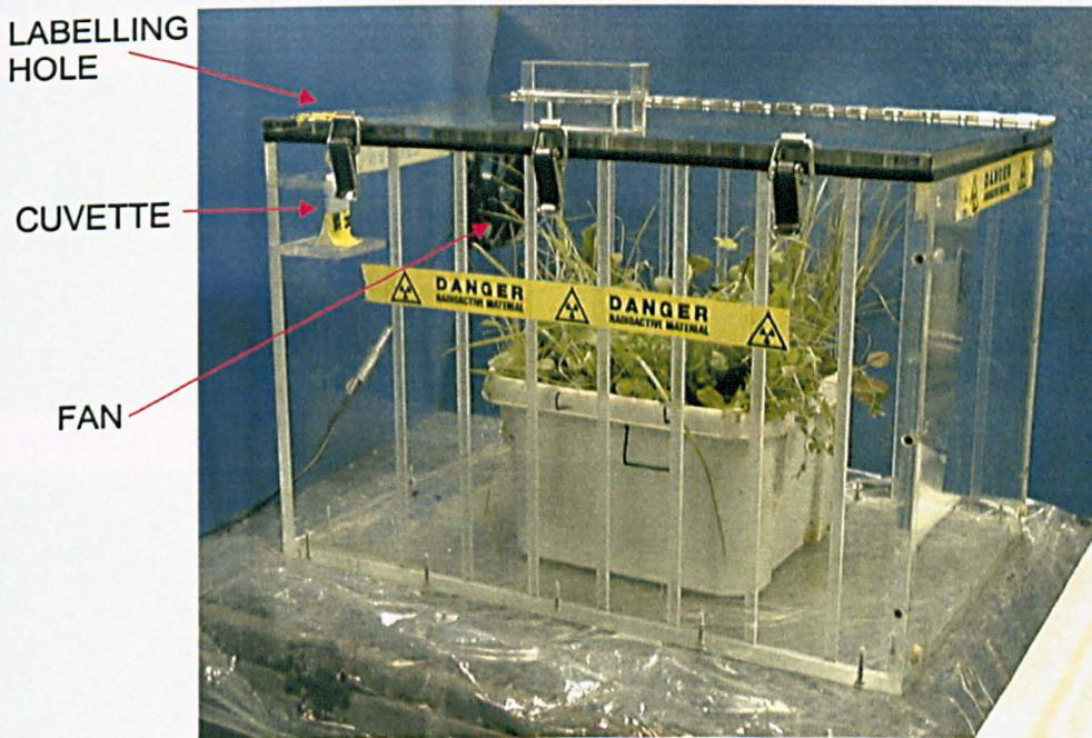
**Fig. 6.2** Labelling chamber containing turf-core system.
