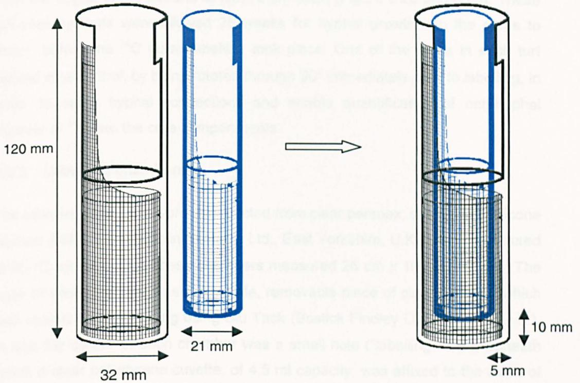
**Fig. 5.1** Diagrams of double-walled hyphal in-growth cores. Two cores (left) made from plastic tubing with windows cut, with sides and base covered by 35  $\mu\text{m}$  nylon mesh, were fixed together to form a core (right) with inner and outer compartments. Cores are shown here with mesh cut away. There was 5 mm between the sides of the inner and outer cores, and 10 mm between their bases.
