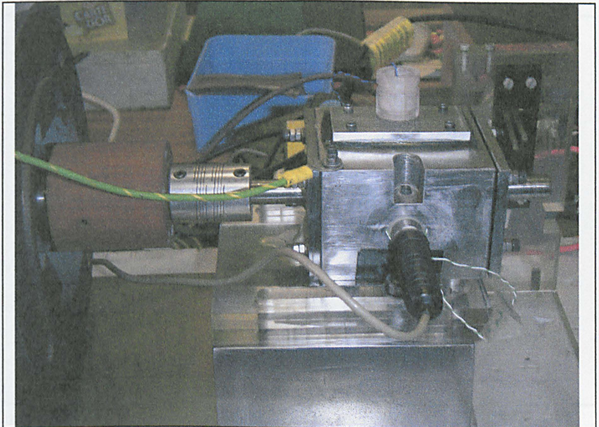
Fig. 5.34: Picture of new ER fluid Rayleigh step bearing rig.
