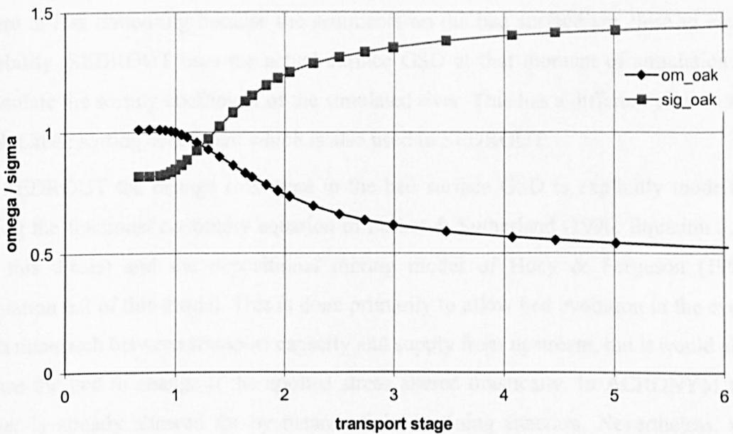
**Figure 7.2:** The Oak Creek straining functions (after Parker, 1990). Transport stage denotes  $\phi'$ . A value of 1 corresponds to the quasi-threshold reference stress for mean diameter. Sig\_oak denotes  $\sigma_o$ , and om\_oak denotes  $\omega_o$ .
