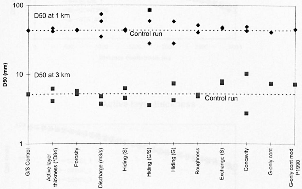
**Figure 7.5:** Output of SEDROUT V.2 sensitivity analysis model runs showing bed surface  $D_{50}$  at time  $T_w$  for various parameters. G and S indicate gravel and sand respectively P1990 denotes the original Parker (1990) bedload transport relation. The figure is best viewed in association with Table 7.2, showing parameter values.
