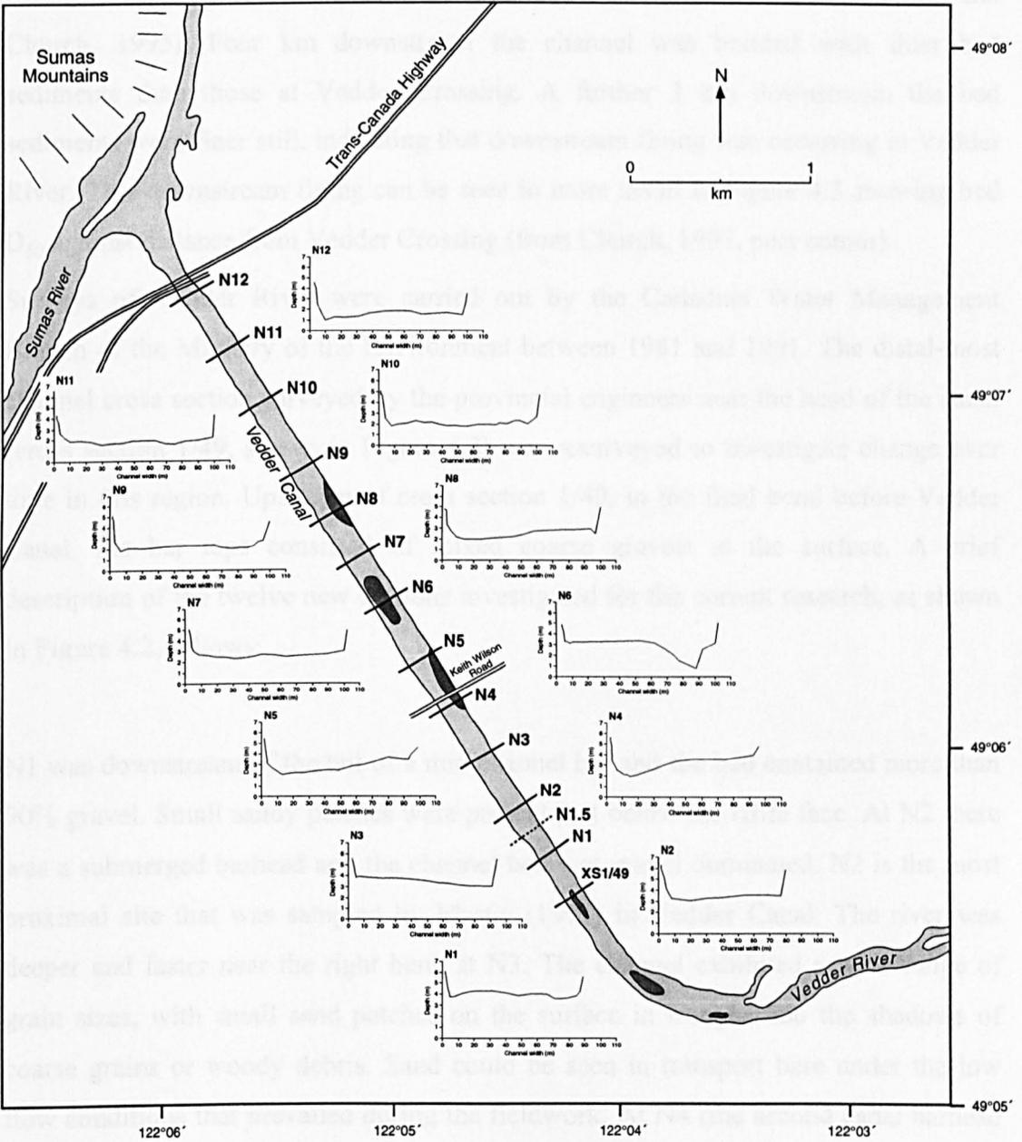
**Figure 4.2:** The gravel-sand transition reach of Vedder Canal in 1998. Positions of cross sections and cross section profiles are plotted. Gravel bars are shown as darker areas in the stream. Flow is from bottom right to top left.
