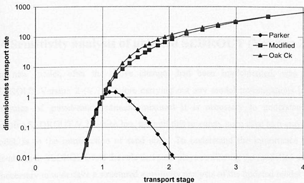
**Figure 7.4:** Behaviour of the modified straining function for mean diameter in a poorly sorted bed ( $\phi$  standard deviation,  $\sigma$ , of 3) compared with the Oak Creek relationship and the Parker (1990) straining function.
