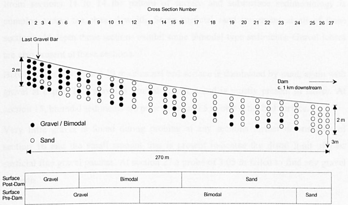
**Figure 5.6:** Simplified one-dimensional diagram of subsurface sedimentology from probing information gathered in the GST reach of Allt Dubhaig. Inferences are made regarding the bed surface sedimentology before and after dam construction.
