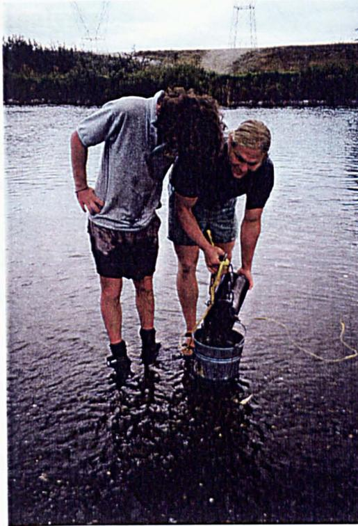
**Figure 4.4:** Pipe dredge used to collect bed surface sediment samples from Vedder Canal.
