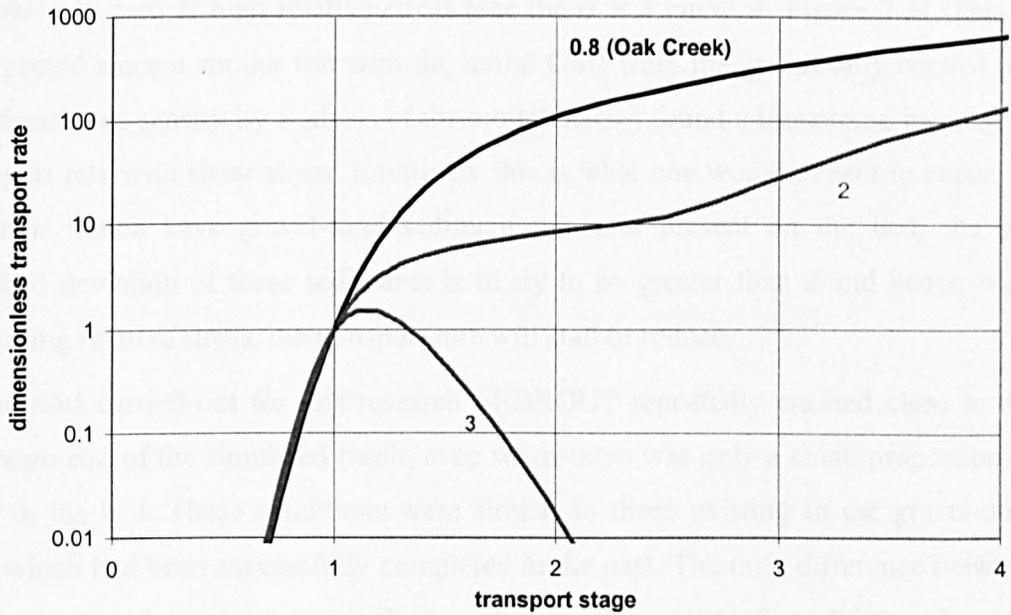
**Figure 7.3:** Behaviour of the transport function  $G(\phi'')$  for the mean diameter in a poorly sorted bed ( $\phi$  standard deviation,  $\sigma$ , of 2 or 3) using the Parker (1990) straining function. The original Oak Creek relationship is also plotted. Transport stage denotes  $\phi'$  and dimensionless transport rate is  $w^*_i$ .
