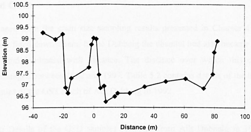
**Figure 5.3:** Cross section 1/49 of at the head of Vedder Canal, mapped in 1998.
