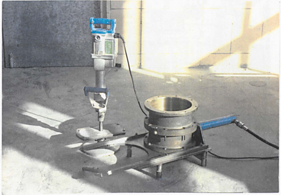
Plate A1 Kango hammer and compaction guide for test series A and B
