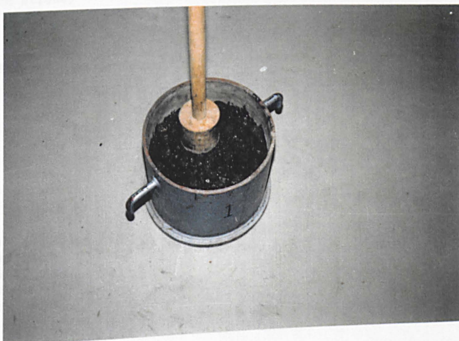
Plate A12 Compaction apparatus used to apply a low compactive effort to test specimens for use in test series D
