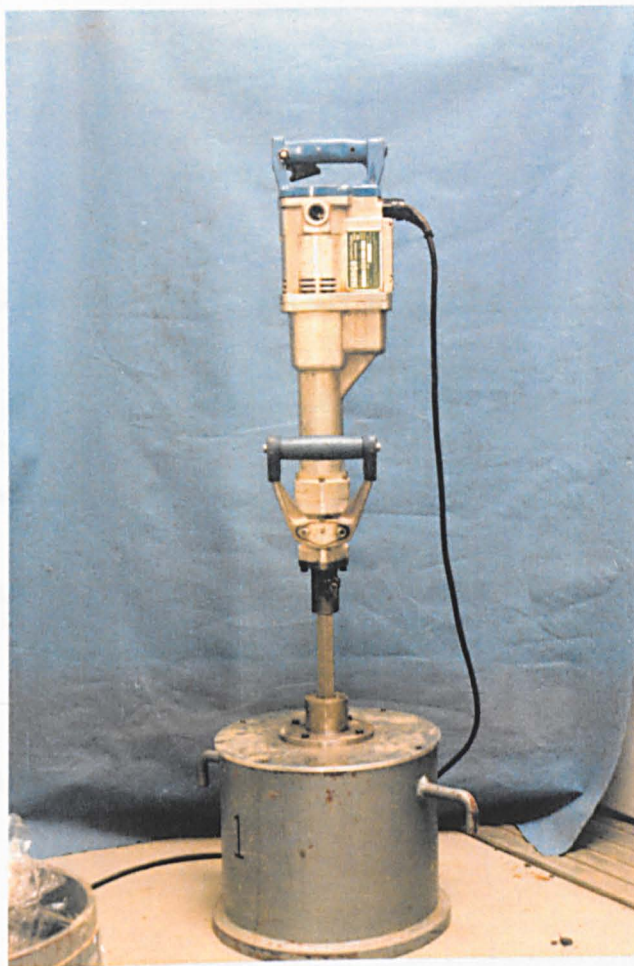
Plate A11 Compaction apparatus used to apply a high compactive effort to test specimens for use in test series D
