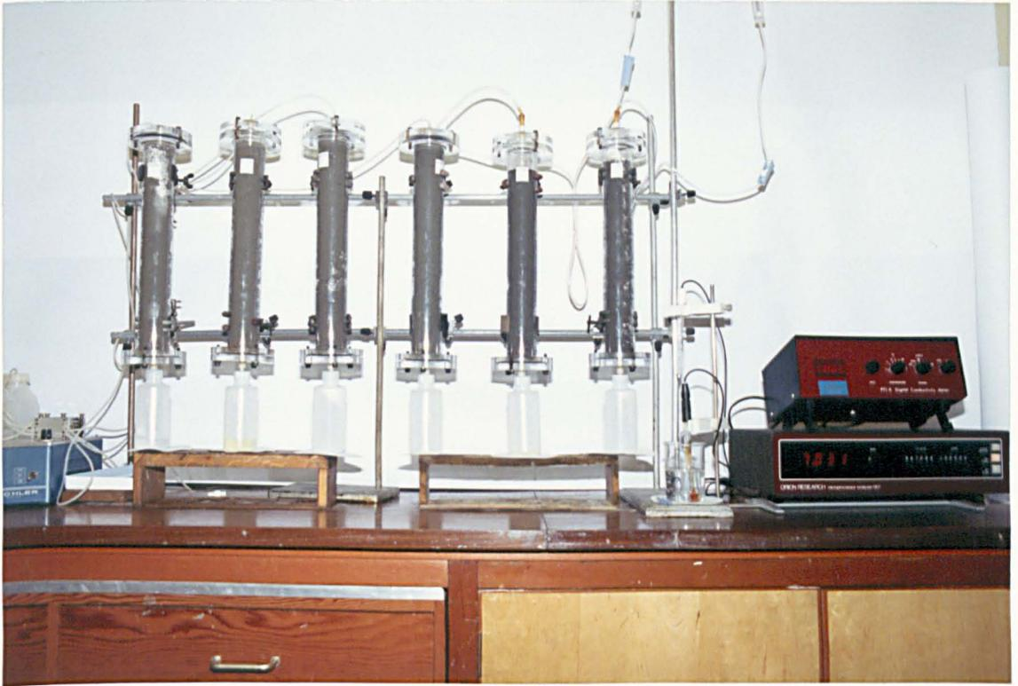
Plate A. Laboratory set-up for column leaching tests
