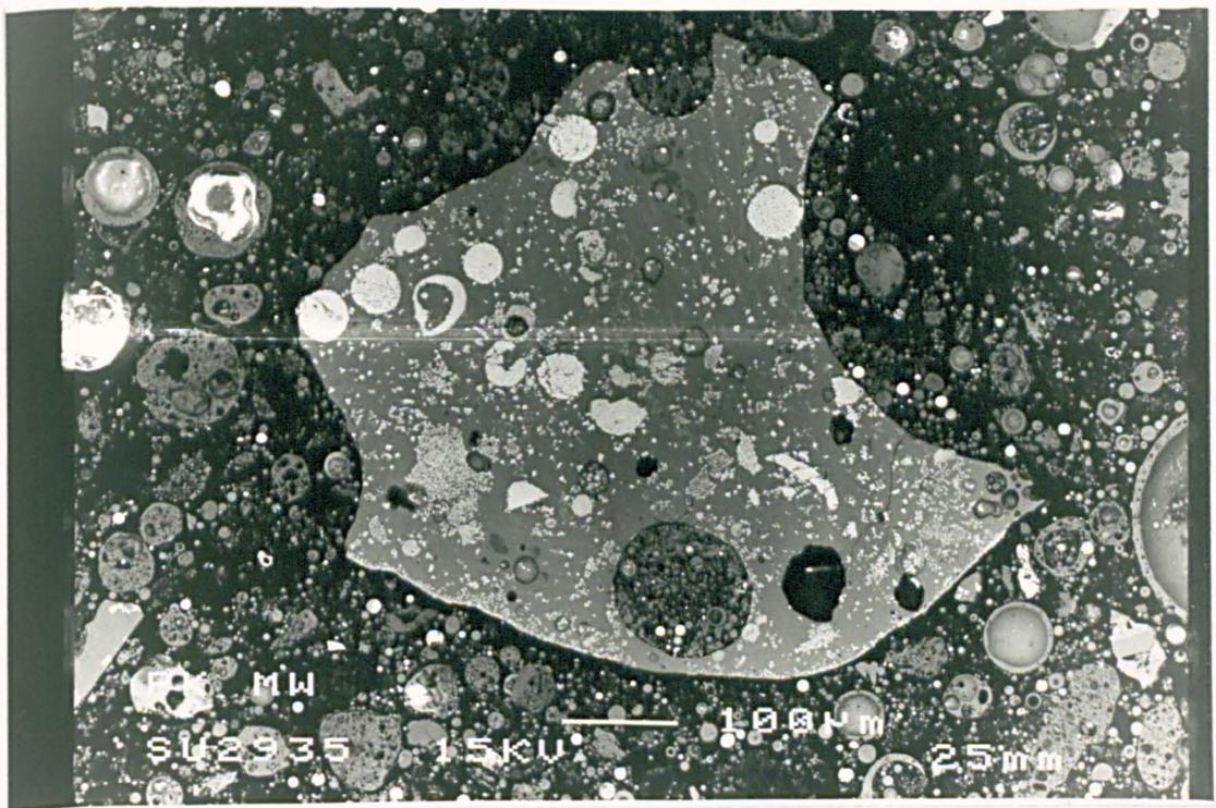
**(c) Iron-rich particle, showing a dendritic structure**
