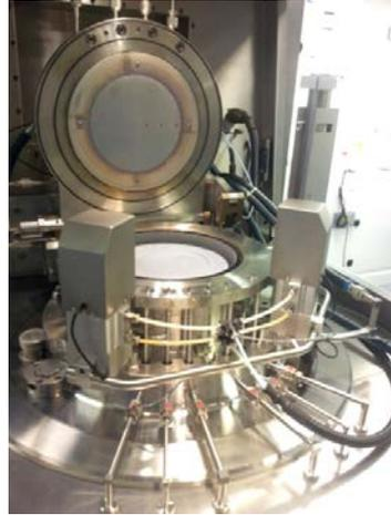
Figure 2.2: Photograph of the inside of a Thomas Swan MOVPE reactor chamber.
