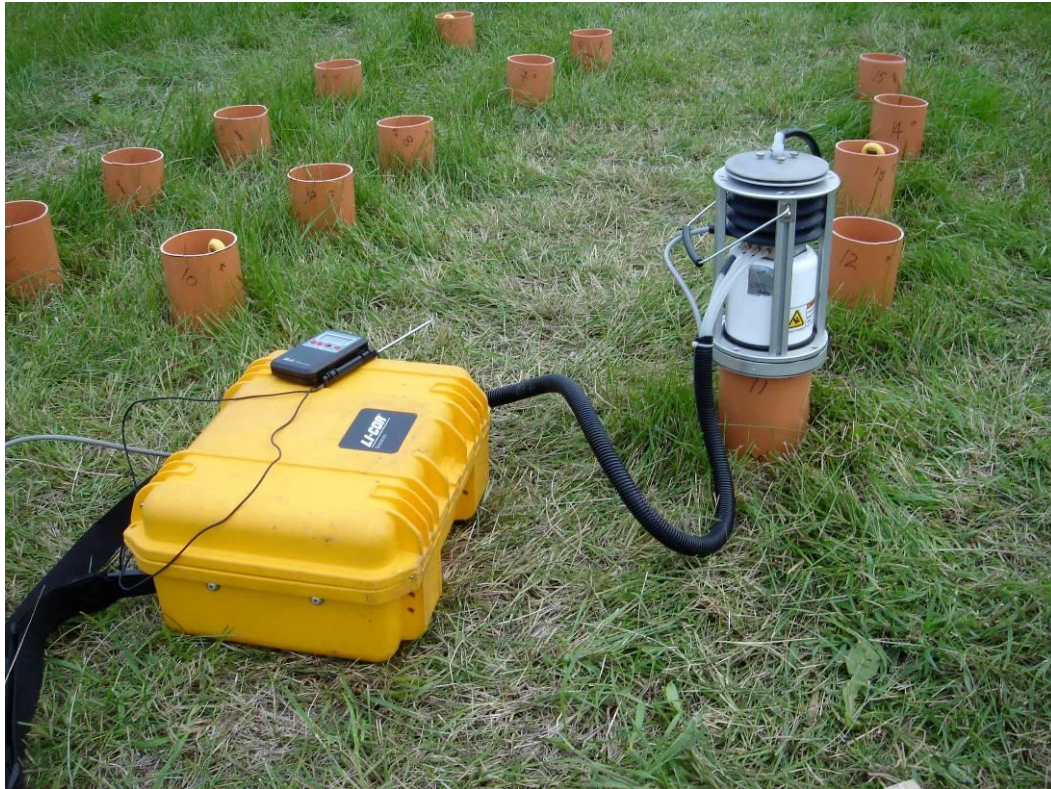
Fig. 5.5 Photograph of pre-treatment CO 2 flux measurement from soil collar number 11 using the IRGA and automatic survey chamber.
