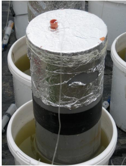
Fig. 3.1 Photograph of a cuvette on top of a peat soil mesocosm ready for CH 4 sampling.
