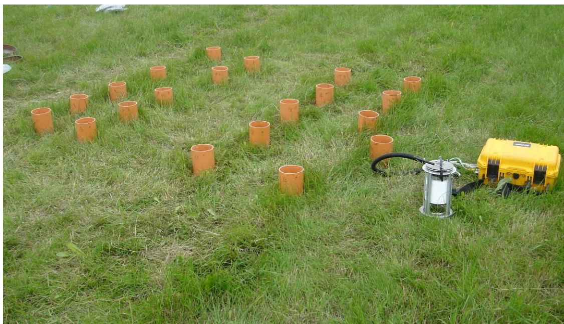
Fig. 5.4 Photograph of the experimental set up at Smáratún. Twenty PVC collars inserted 5 cm into the soil with the IRGA and automatic survey chamber.
