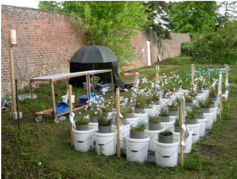
Fig. 2.3 Photograph of the experimental setup in the walled garden at the University of York. Intact peat mesocosms were placed in buckets under natural conditions for the duration of the experiment.
