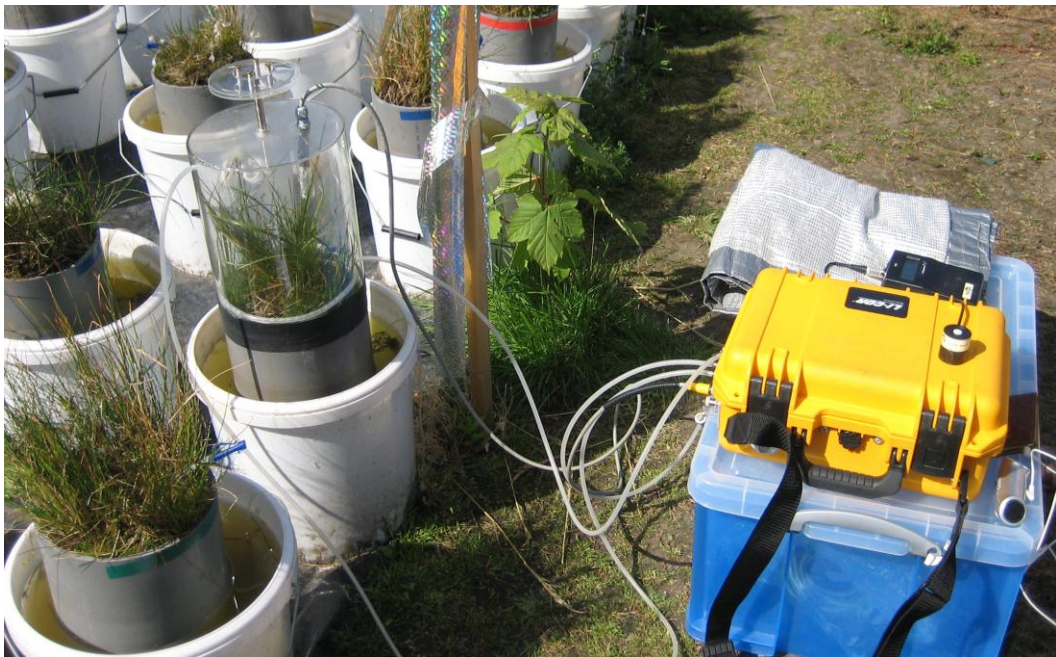
Fig. 3.2 A transparent chamber attached to the IRGA to measure mesocosm CO 2 flux in light.
