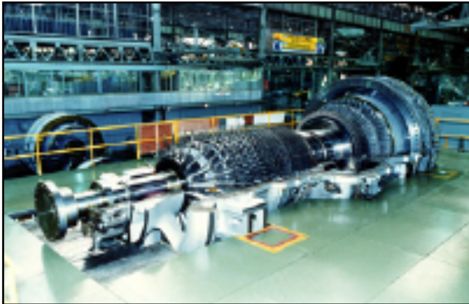
Figure 7-7 Ratchaburi gas-fired gas turbine combined cycle, GTCC (Ikuno, 2005). The figure shows of a typical gas turbine engine. Air is compressed by the fan blades as it enters the engine, and it is mixed and burned fuel with fuel in the combustable section. The hot exhausted gases provide forward thrust and turn the turbine the turbines with drive the compressor fan blades.
