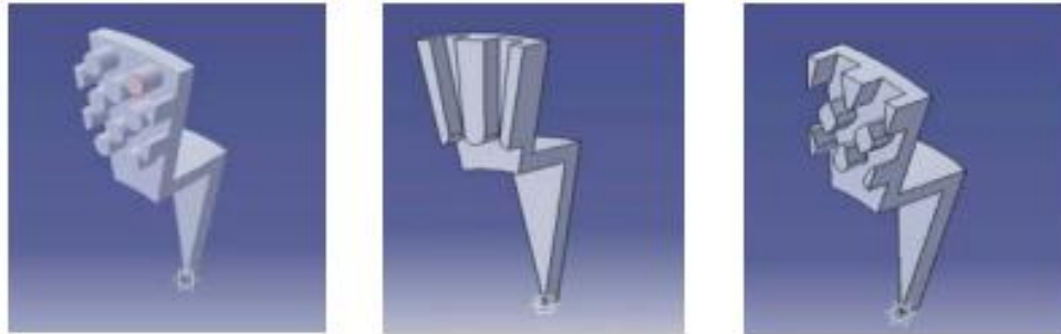
Figure 2-10: Circular pillar (CP) vane, modified taper radial (MTR) vane and diamond pillar (DP) vane (Raj et al., 2014)
