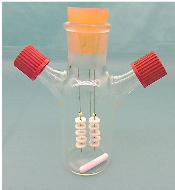
Figure 2. 1. The dynamic culture of BCs in spinner bioreactor. Figure shows ROS cells–seeded HA/TCP scaffolds threaded in spinner before the addition of CDMEM–LAA and transferring to the incubator.
