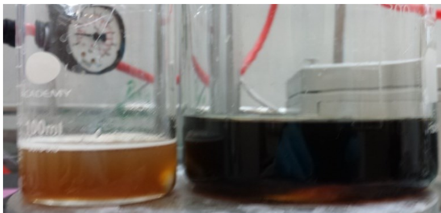
Figure 82. Stripped leachate (left) compared to untreated leachate (right). The stripped leachate was processed in mode 1 and there is a noticeable colour change.
