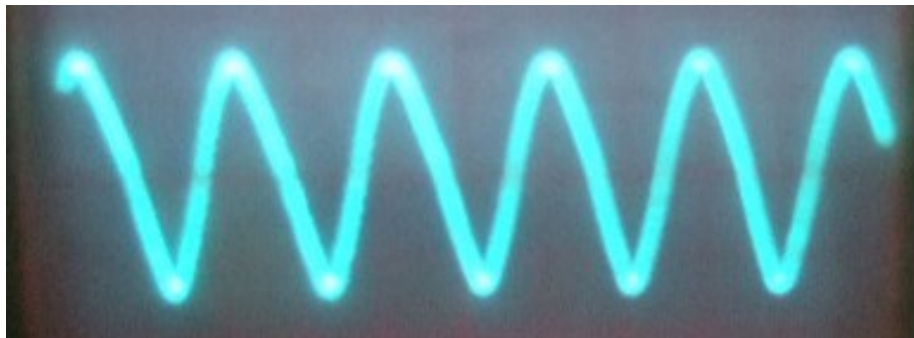
Figure 7 Oscillatory output using the small capacitive volume (3 cc) : Supply pressure 0.5 barg, 275 Hz, flow = 47 slpm( Tippetts, 2014)
