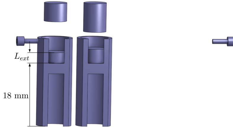
Figure 5.36: Simulation model setup for the estimation of external coupling tunability.
