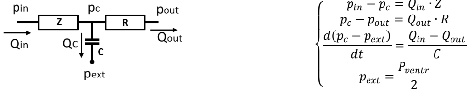
Figure 2.5: 0D model of the coronary branches, using an external pressure on the capacitor.
