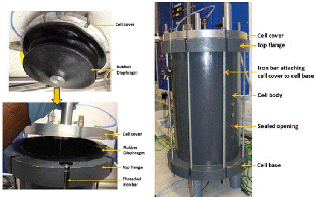
Figure 3.44: Attaching the cell cover to the test chamber
