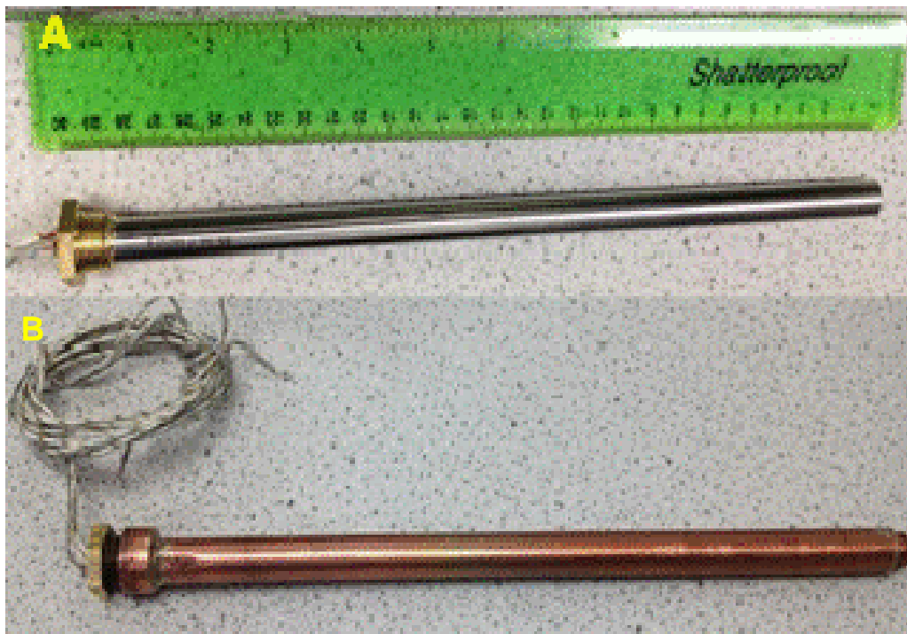
Figure 3.15: Cartridge heater and cartridge heater in copper pipe
