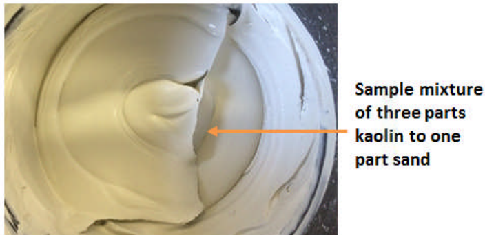
Figure 4.5: Photo showing sample mixture of three parts of kaolin to one part of sand in the test chamber
