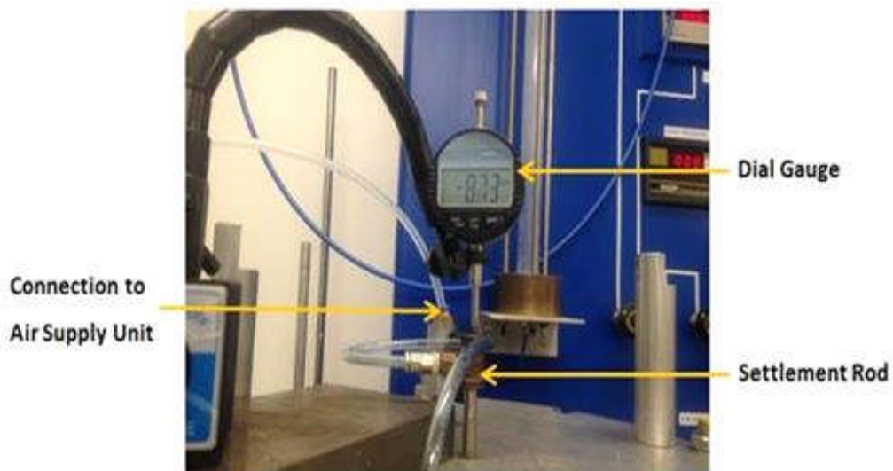
Figure 4.11: Settlement dial-gauge set up to monitor progress of consolidation in sample
