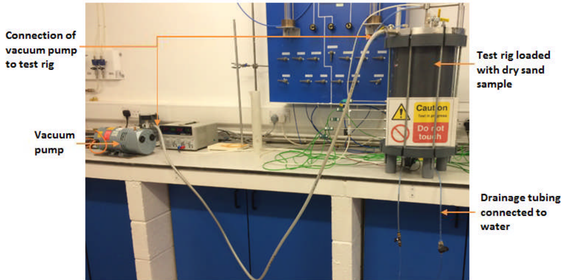
Figure 4.9: Photo showing the process of preparation of saturated sand sample where water is connected to the rig through the drainage tubing and the vacuum pump is connected to the rig to suck out air from the sample while drawing water into the sample
