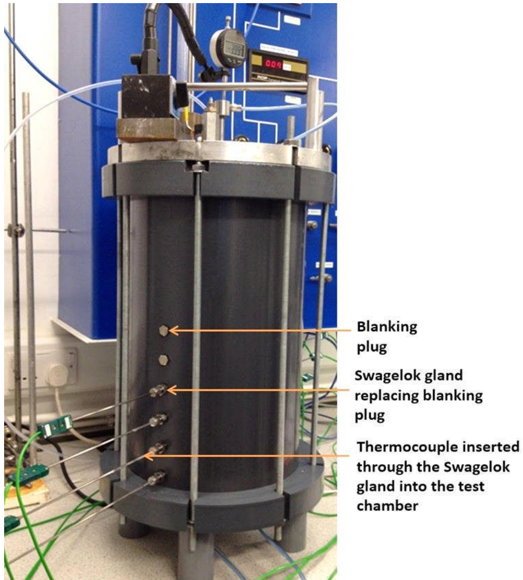
Figure 4.12: The blanking plugs are replaced with Swagelok gland for insertion of thermocouples
