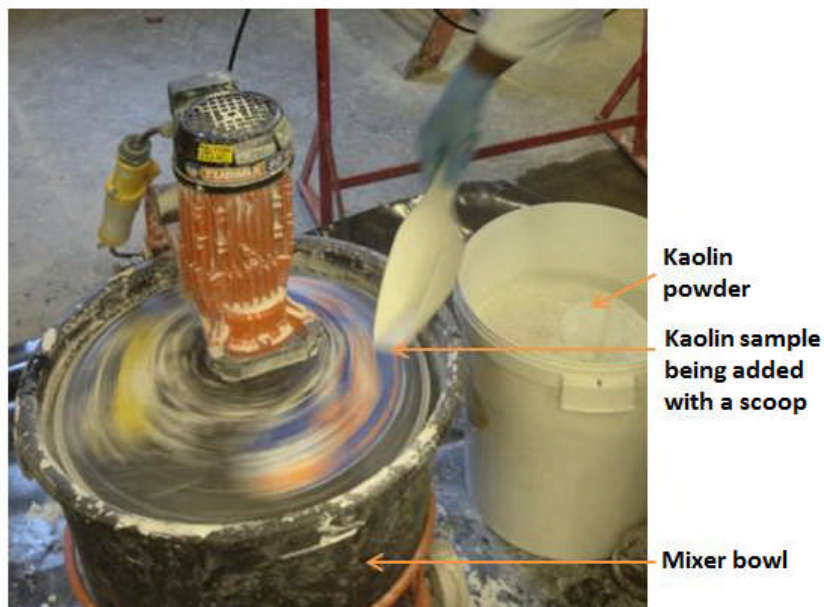
Figure 4.3: Photo showing kaolin sample mixing process where kaolin powder is being added to the distilled water in the mixer bowl
