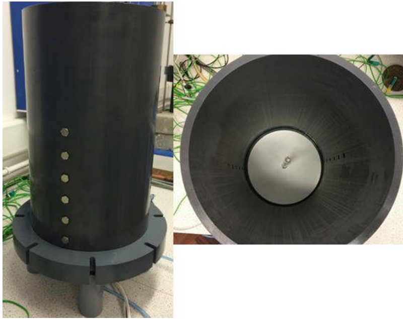
Test Chamber mounted on cell base and inside view showing centrally placed heater
