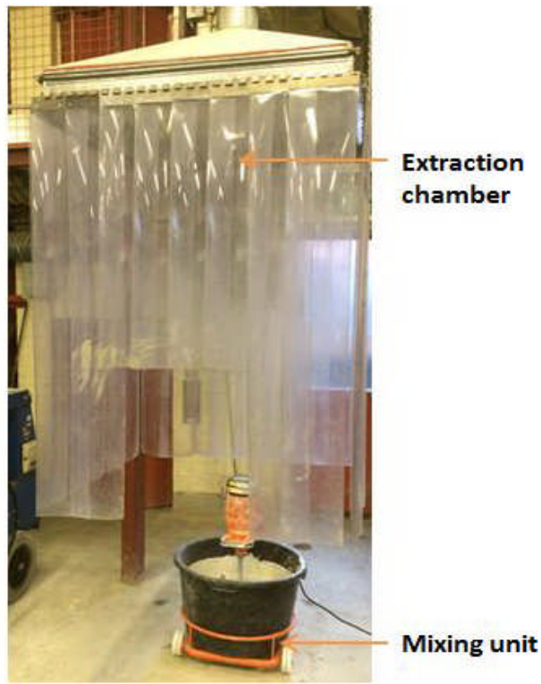
Figure 4.2: A mixing unit set up inside an extraction chamber for mixing samples
