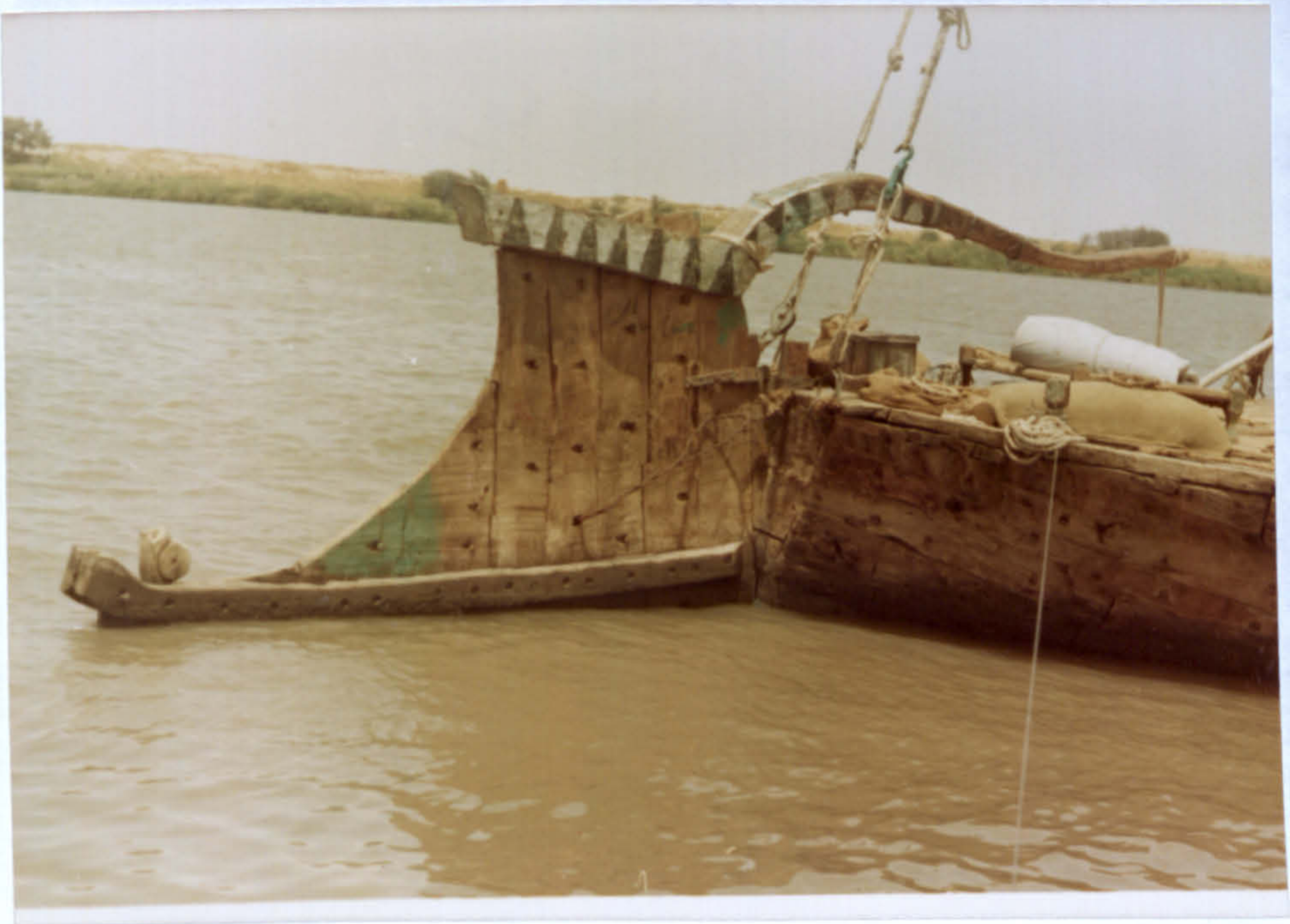
Plate 15. The rudder and its parts, the tiller, the rudder blade and the rudder head. Loops.
