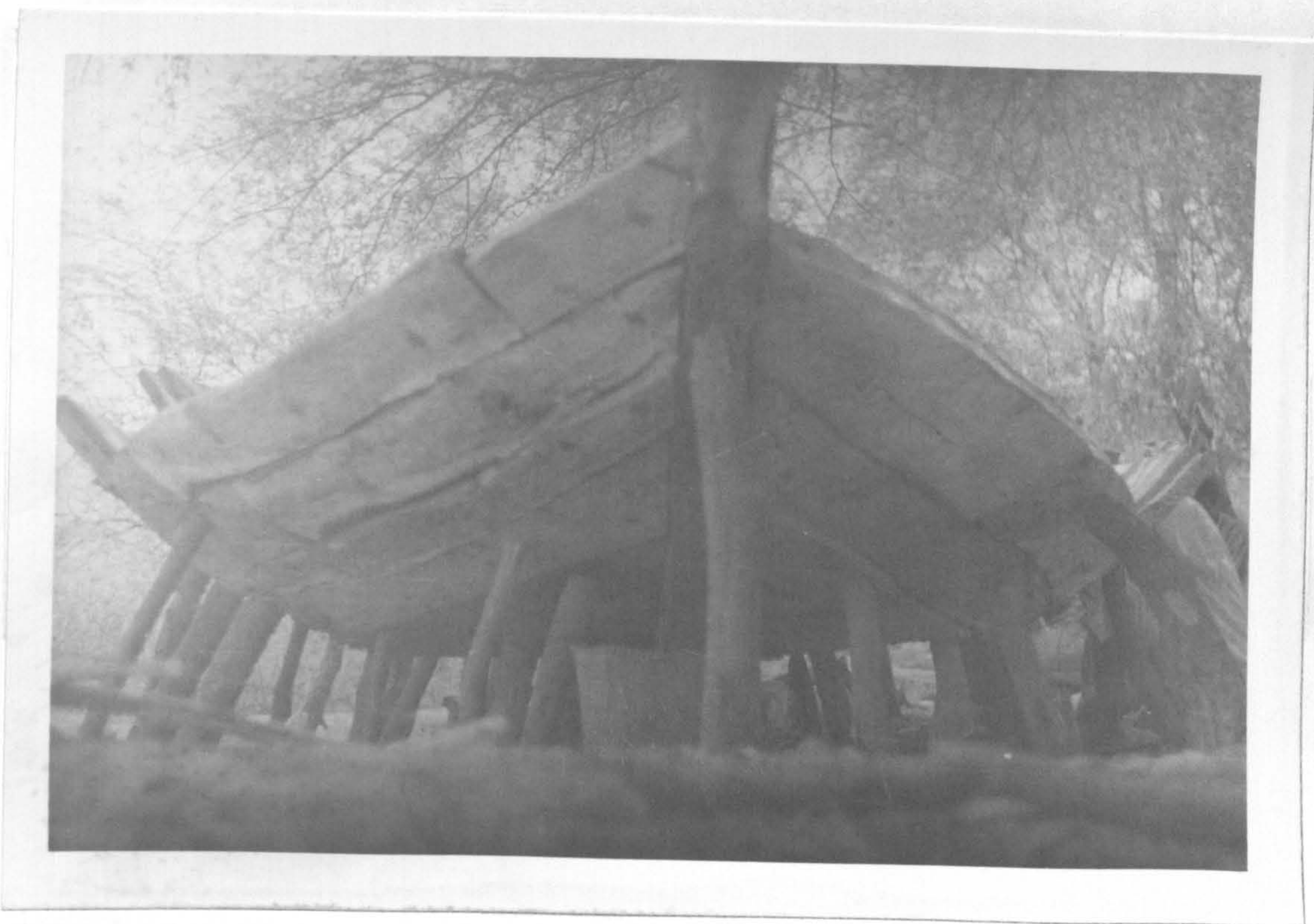
Plate 12. The boat on the stocks during the process of its building.
