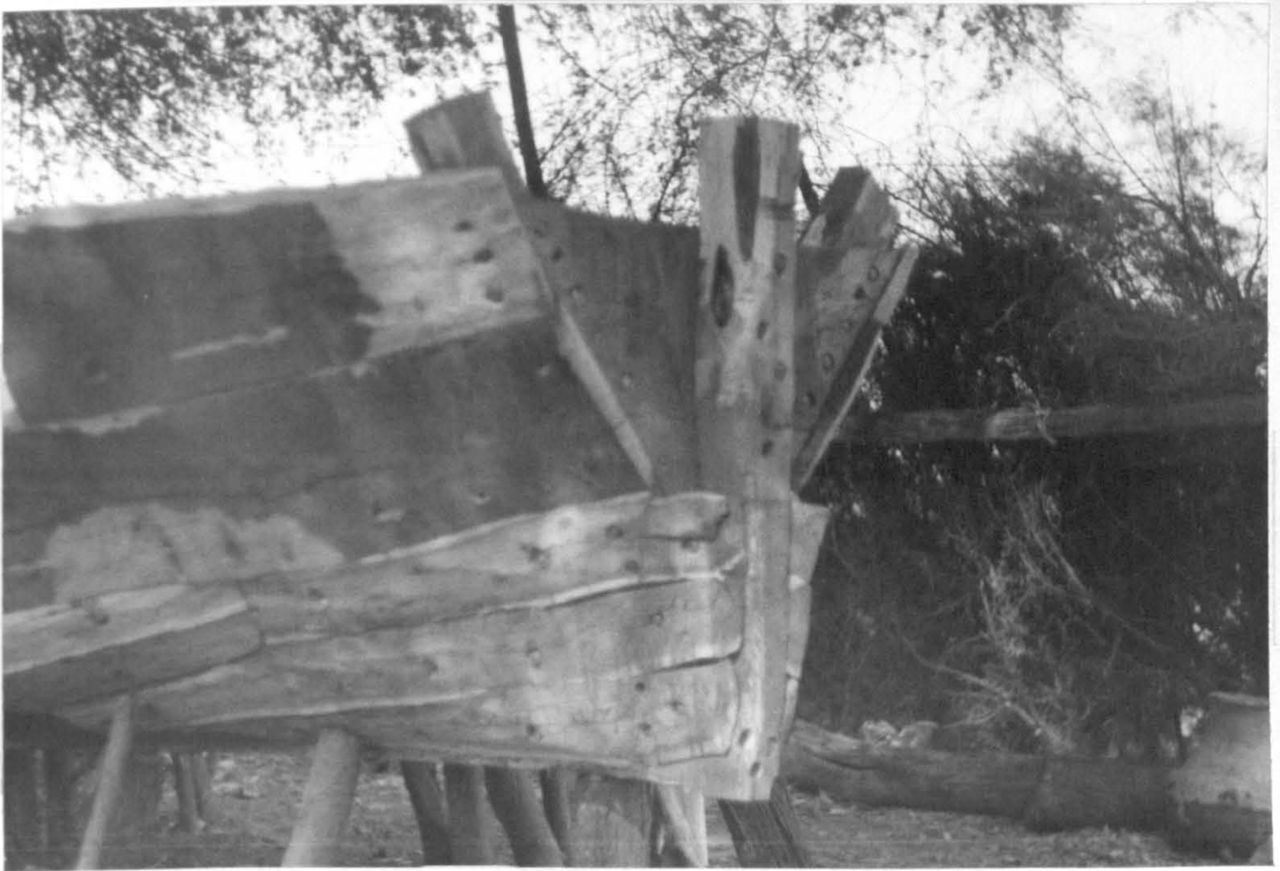
Plate 10. The oval pits on the planks where the heads of the spikes recess to make the boat countersunk.
