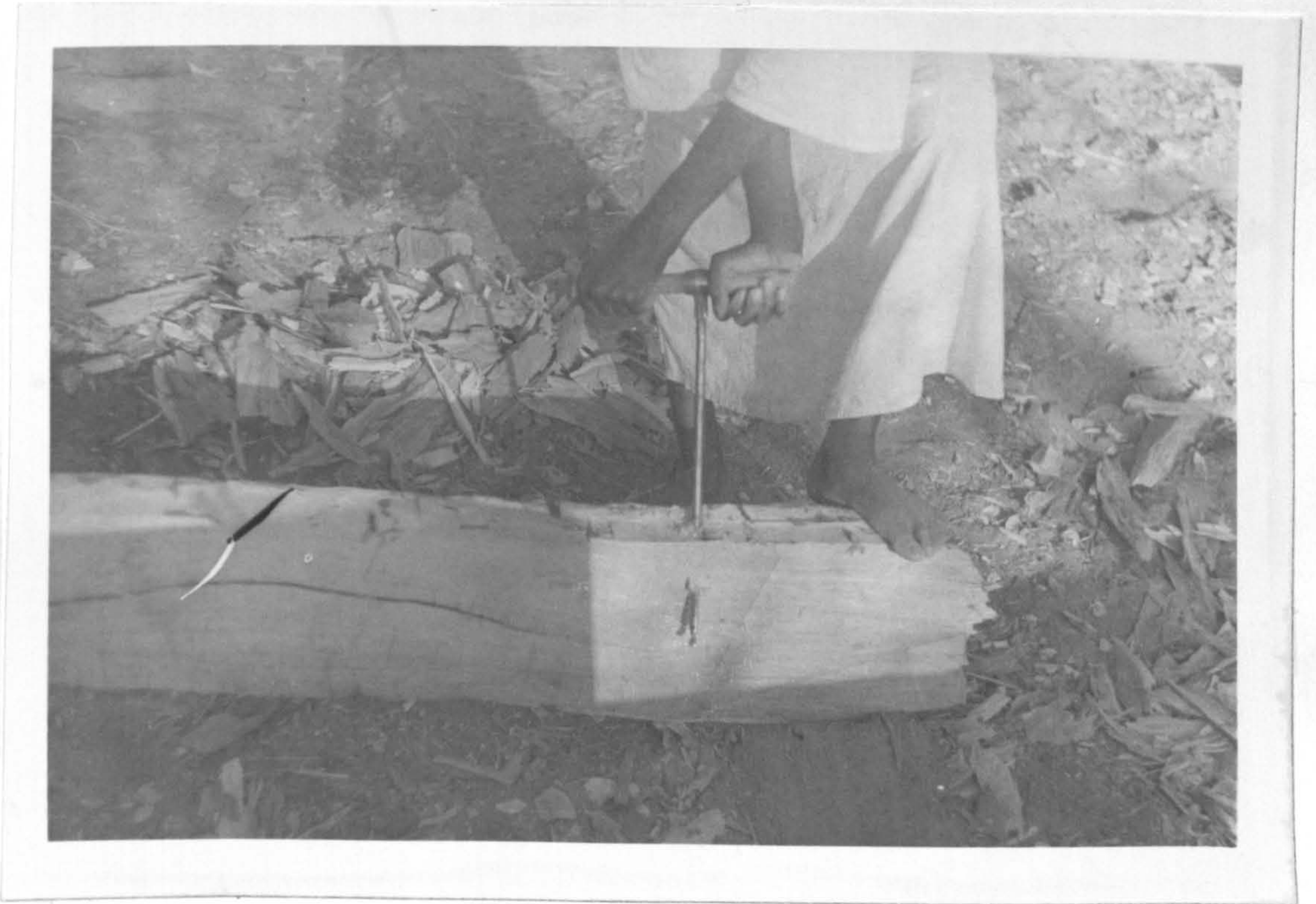
Plate 9. The craftsman using the auger drill to open holes for the spikes.
